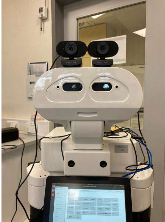
Figure 3.4: Tiago++ with webcams.
