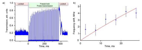
Figure 5.12: Temperature dependent drift of the frequency of the resonator mode. (a) The resonator is first frequency stabilized on resonance. Then, the response of the resonator to a sudden change in power is probed for about 450 ms before turning on the frequency stabilization again. (b) Exponential fit to the data in (a) with a thermal relaxation time constant of  $\bar{\tau}=105$  ms.  $Q_{\rm crit}=4.2\times10^7$ , Input laser power = 50 nW.
