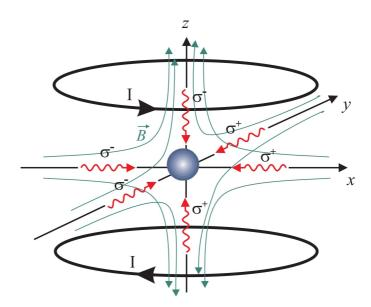
Figure B.5: Sketch of the magnetic fields and light fields in a 3D MOT. Current, I, flows in two coils in anti-Helmholtz configuration and produces the magnetic field  $\vec{B}$ . Three pairs of counter-propagating beams are arranged to all be mutually perpendicular, to have circular polarization, and are red-detuned from the atomic transition. The beams in the xy-plane have left-handed helicity while the beams in the z-axis have right handed helicity. Reproduced from Ref. [57].
