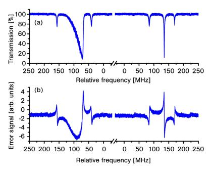
**Figure 5.7: Thermal bistability of a resonator mode.** (a) With decreasing frequency (left), the transmission of the carrier appears broadened, and with increasing frequency (right), the transmission of the carrier appears narrowed. Correspondingly, the error signals are also distorted, see (b).
