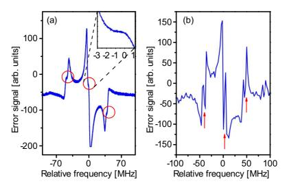
**Figure 5.8:** Mode splitting in two different resonator modes. (a) Resonances with small mode-splitting cause small plateaus (highlighting circles) in the PDH error signal near critical coupling. (b) Under-coupled resonances with large mode-splitting result in sign changes of the slope (arrows) meaning that the phase changes non-monotonically.
