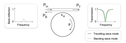
Figure 2.5: Model of a coupling fiber and single-mode WGM resonator. The left fiber port  $(P_{\rm in})$  is taken as the input port which couples evanescently to the resonator. The transmission and back-reflection characteristics of each port are sketched for the cases of traveling and standing wave cavities.
