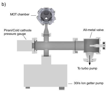
**Figure 4.4: Overview of the lower vacuum chamber.** (a) Atoms trapped and cooled in a MOT in the spherical-cube chamber are vertically launched through a differential pumping tube to the science chamber. (b) Cross-section through the setup showing the layout of the ion pump, all-metal right angle valve connected to a turbo pump, and pirani/cold cathode pressure gauge for measuring pressures down to  $3 \times 10^{-9}$  mBar. Adapted from Ref. [88].
