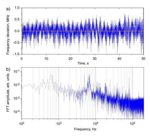
**Figure 5.10: Stabilization of an ultra-high** Q-factor bottle mode in vacuum. (a) Frequency deviation: when the resonator is stabilized to the laser, which is in turn stabilized to the  $D_2$ -transition of  $^{85}$ Rb using a Doppler-free spectroscopy setup, fluctuations are visible around the setpoint of the transmitted power. The rms value of these fluctuations is 418 kHz and is marked with dashed lines. (b) FFT spectrum of the frequency deviations in (a).
