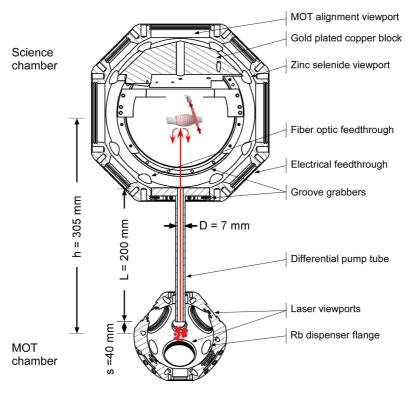
**Figure 4.3: Cross-section through the vacuum apparatus.** Rubidium is cooled in a magneto-optical trap in the lower chamber. The atomic cloud is then launched through a differential pumping tube into the upper chamber where it reaches the resonator at a height of around 305 mm.
