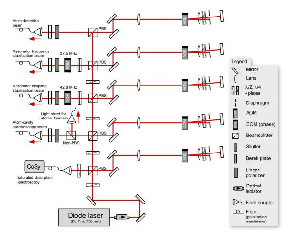
Figure 4.17: Laser setup for probing the atom-resonator interaction and stabilizing the resonator and coupling fiber. AOMs are used to control both the power and frequency in each beam, while EOMs are used in a Pound-Drever-Hall resonator stabilization scheme (see main text of next chapter).
