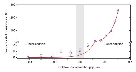
Figure 3.6: Red-shift of optical resonance frequency as a function of coupling fiber loading. The solid line is an exponential fit arising from the exponential dependence of the overlap between the resonator and coupling fiber modes. Error bars:  $\pm 2$  MHz.
