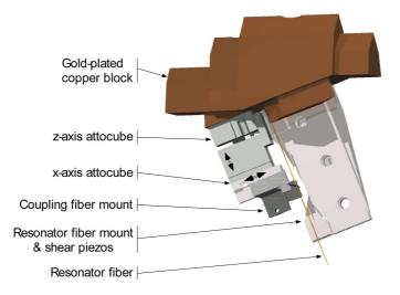
**Figure 4.13: Side-view of the fiber translation stages and the resonator setup.** The coupling fiber axis is perpendicular to both the resonator fiber axis and image plane. Only the translation stages for one coupling fiber are shown for clarity.
