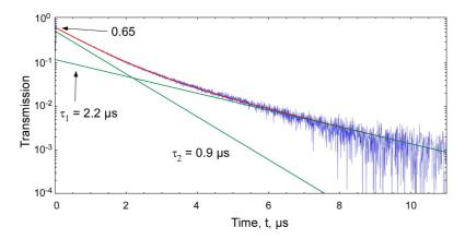
Figure 7.2: Transmission time dependence after FPGA trigger using the single atomdetection scheme. Zoom of the transmission decay after atom detection at  $t=0~\mu s$  in Fig. 7.1 (b) and with a transmission offset of 2.6% subtracted. The red line is a fit to the data using the sum of two exponentials (green lines) with time constants  $\tau_1 = 2.2~\mu s$  and  $\tau_2 = 0.9~\mu s$ . Bin width: 4 ns.
