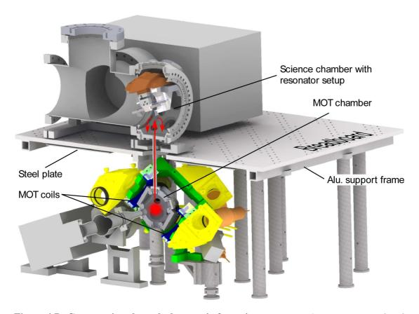
**Figure 4.7: Cross-section through the atomic fountain apparatus.** Atoms are trapped and cooled in the lower MOT chamber and subsequently launched to the upper science chamber where the resonator setup is mounted. The opto-mechanics and magnetic coils necessary for the MOT are highlighted. Adapted from Ref. [88].
