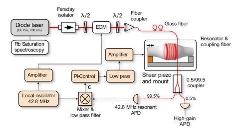
**Figure 5.2:** Schematic of the Pound-Drever-Hall stabilization setup and resonator geometry. Frequency sidebands at 42.8 MHz are generated in the laser beam spectrum by phase modulating it with an electro-optic modulator (EOM). For clarity, the scale of the resonator is exaggerated with respect to the resonator mount.
