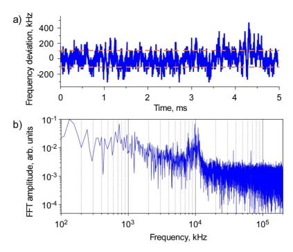
Figure 5.5: Frequency noise of an ultra-high Q-factor bottle mode. (a) When the resonator is stabilized to the laser, fluctuations are visible around the setpoint of the transmitted power. The rms value of these fluctuations is 206 kHz and is marked with dashed lines. (b) FFT of the frequency fluctuations. The data is measured with 2–3  $\mu$ W of launched power. The measurement in (a) is measured with the high-gain APD.
