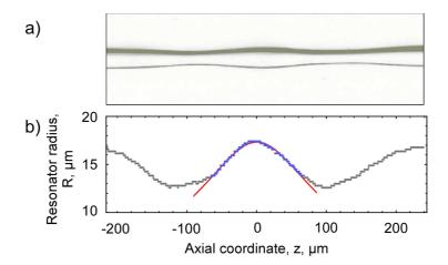
Figure 3.2: Reconstructing the profile of a bottle microresonator. (a) Microscope picture of a bottle microresonator with the edges highlighted in grey. (b) The reconstructed radius profile of a typical resonator used in this work agrees well with a parabolic fit (red) (see Eq. (1.25)) in the central region around z=0. The fit yields  $R_0=17.4~\mu m$  and  $\Delta k=0.012~\mu m^{-1}$ . Measurement tolerance:  $R_0:\pm 2.0~\mu m$ ,  $\Delta k:\pm 0.001~\mu m^{-1}$ .
