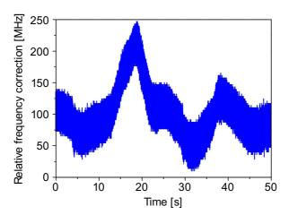
**Figure 5.6: Slow frequency drifts of the stabilization scheme.** When the resonator is stabilized to the spectroscopy-stabilized laser, the correction signal sent to the piezo is proportional to the compensated frequency drift of the resonator. The signal is measured before the 4 kHz low pass filter.
