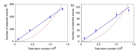
Figure 7.5: Dependence of the number of detected atom-resonator coupling events for different atomic densities. (a) Single detection scheme: single-atom coupling events follow a linear dependence (solid line) while, for comparison, two-atom coupling events follow a quadratic dependence (dashed line). (b) The number of observed events using the double atom-detection scheme similarly follows a linear dependence.
