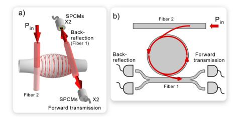
**Figure 7.11: Coupling setup using two fibers.** (a, b) Light in fiber 2 (also labeled as fiber 2 in the fiber network in Fig. 6.1) is coupled into the empty resonator which itself couples to fiber 1. Fiber 1 is critically coupled to the resonator and couples out  $\sim 50\%$  of the light, while fiber 2 is weakly coupled to the resonator and couples in (out) 10% of the pump (resonator) light.
