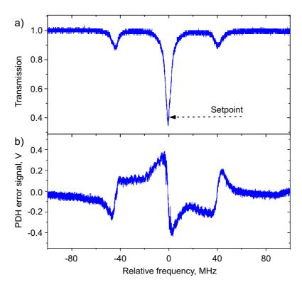
Figure 5.9: Ultra-high Q-factor bottle mode in a vacuum of  $2 \times 10^{-9}$  mBar. The mode line-shape (a) reveals a linewidth of 5.4 MHz ( $Q_0 = 1.4 \times 10^8$ ) which is calibrated using sidebands as frequency markers. The corresponding PDH error signal is shown in (b).
