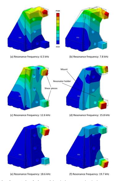
**Figure 5.3: Finite element simulations** of the six lowest mechanical resonance frequencies of the resonator holder device. The resonator fiber (not shown) is held between two shear piezos that are glued to a resonator holder which is in turn mechanically attached a triangular mount, of which both are made of aluminum. The amplitude of the relative motions is indicated by color coding and is also graphically displayed (displacement is exaggerated).
