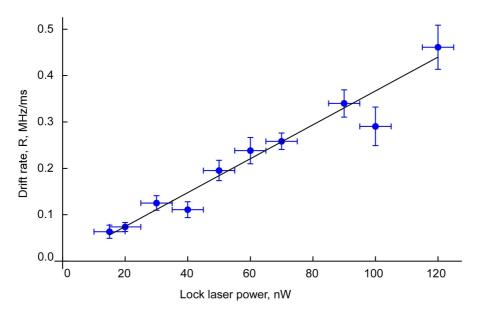
**Figure 5.11: Dependence of the drift rate of a resonator mode on lock laser power.** Increasing the power causes the absorption and therefore the drift rate to increase linearly.
