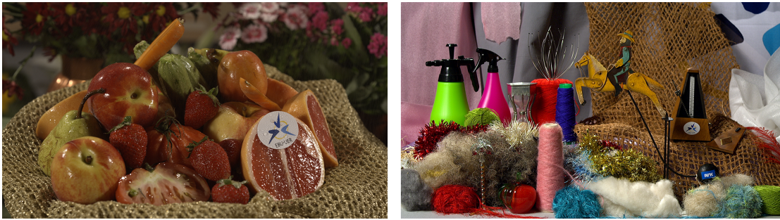
Figure 6.3: UHD-1 (left) and HD (right) test sequences as provided by the EBU. Both sequences represent high-quality raw video captured from professional camera equipment.
