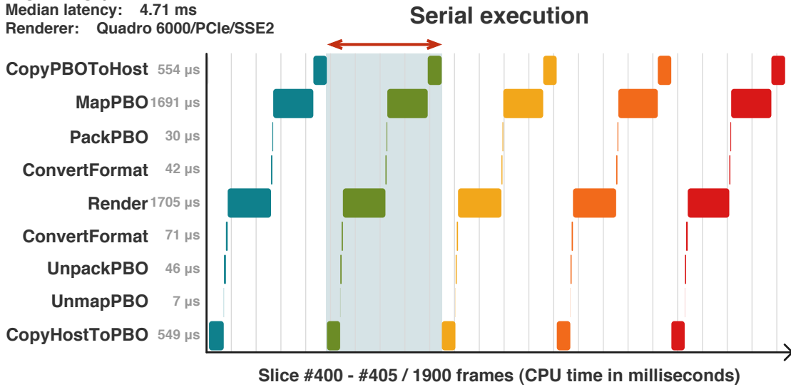
(a) Base configuration. All stages are executed serially. The highlighted area shows how each processing for a single frame is executed sequentially. Used configuration: [A3, B1, C1, D1, E6, F3, G a3,b2,d2 ] (see Figure 6.1).
