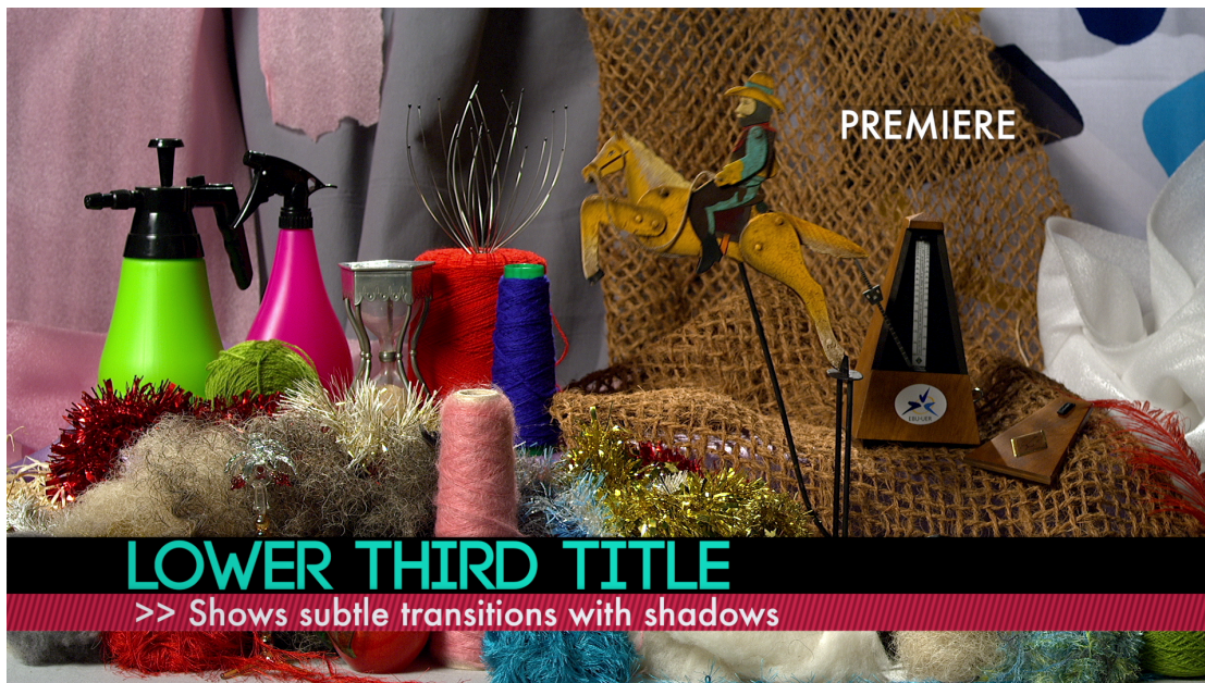
Figure 4.8: The demo renderer blends the logo and the lower-third images on top of the original video material. Image appearance is animated using ease-in and ease-out curves. The image in the background is a single frame of the EBU 1080P test sequence [4].
