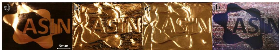
Figure 30: Prepatterned graphene; a) an inverse pattern that is printed in marker ink on a copper foil; dark (inked) areas will not grow graphene, bare copper will; b) the same foil after CVD growth; c) after mild sonication and d) graphene pattern transferred to SiO<sub>2</sub>/Si wafer
