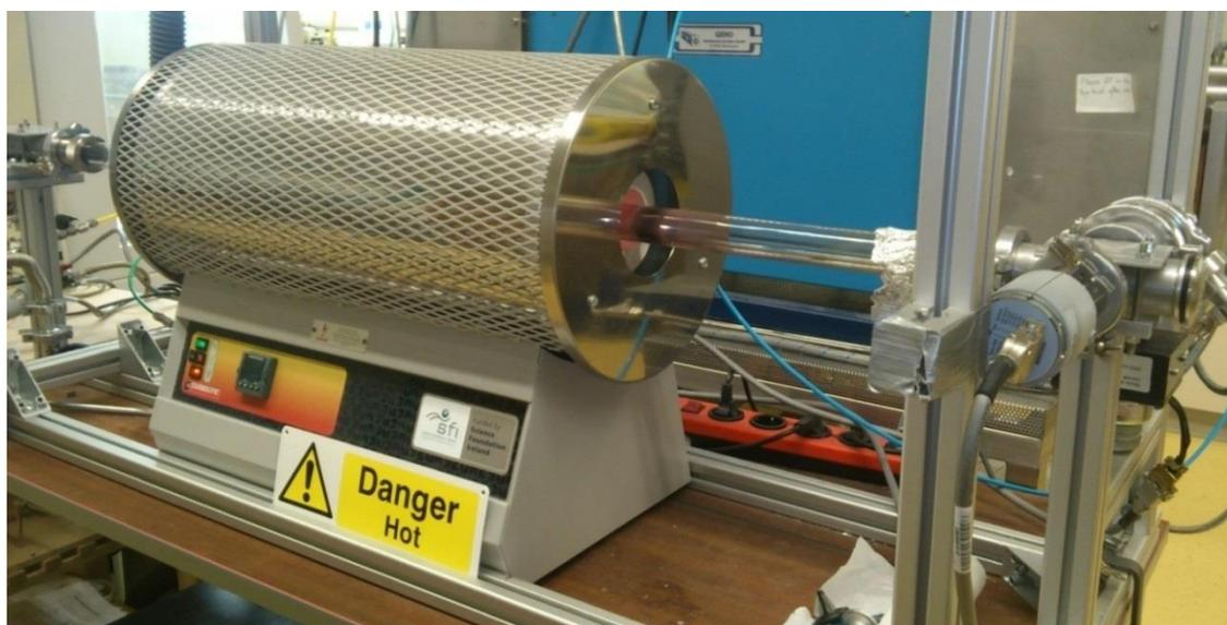
Figure 13: Carbolite furnace for high temperature CVD growth
