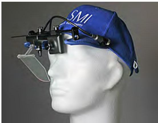
Figure 4.8: Commercial head mounted Eye Tracking System - SMI IVIEW X HED [SMI - Senso Motoric Instruments, 2013a]
