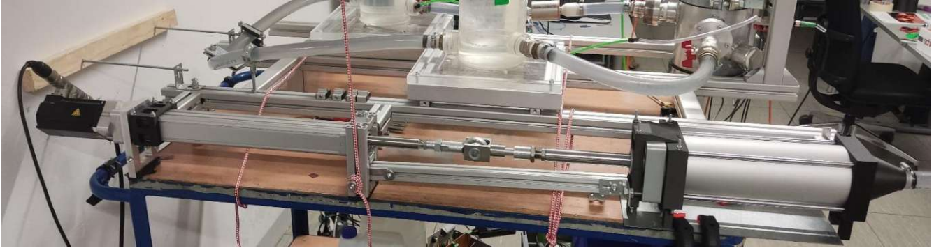
Figure 3- 5 Representation of Motor – Electric Cylinder – Pneumatic Cylinder Assembly
