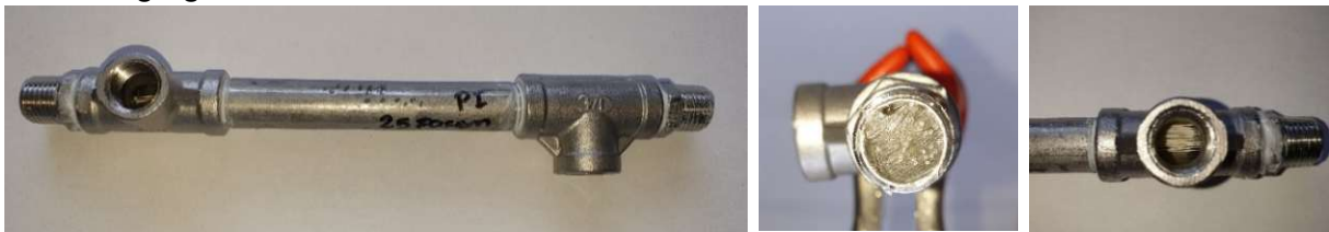
Figure 30: Module of 25 hollow fibres; complete module (far left), view from the lumen (centre) and view from the shell side (far right)
