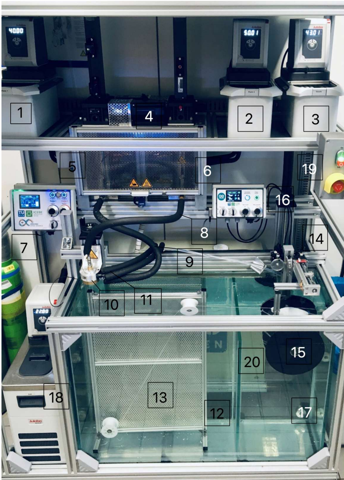
Figure 29: The spinning equipment for the production of hollow fibre membranes: convective thermostats for the dope solution (1), for the bore fluid (2) and the spinneret (3), motors and gearbox for the pumps (4), dope solution pump (5), bore fluid pump (6), pump regulation (7), bore fluid supply pipe (8), polymer supply pipe (9), spinneret (10), spinneret heating pipes (11), coagulation bath (12), fibre with a deflection roller (13), take-up conduction (14), take-up winder drum (15), take-up regulation (16), wash bath (17), convection thermostat for the baths (18), emergency switch (19), safety and electrical box of the equipment (20).
