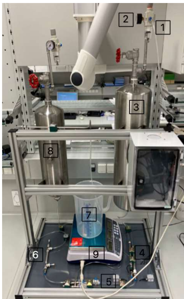
Figure 31: The ultrafiltration unit (left) pressurized air connection (1), pressure indicator (2), feed tank (3), flow indicators (4), needle valves (5), membrane module (6), permeate tank (7), extra tank for a feed (for dead-end configuration)/retentate tank (8), weighing scale (9); flow chart of the ultrafiltration unit built to determine pure water permeance (right)
