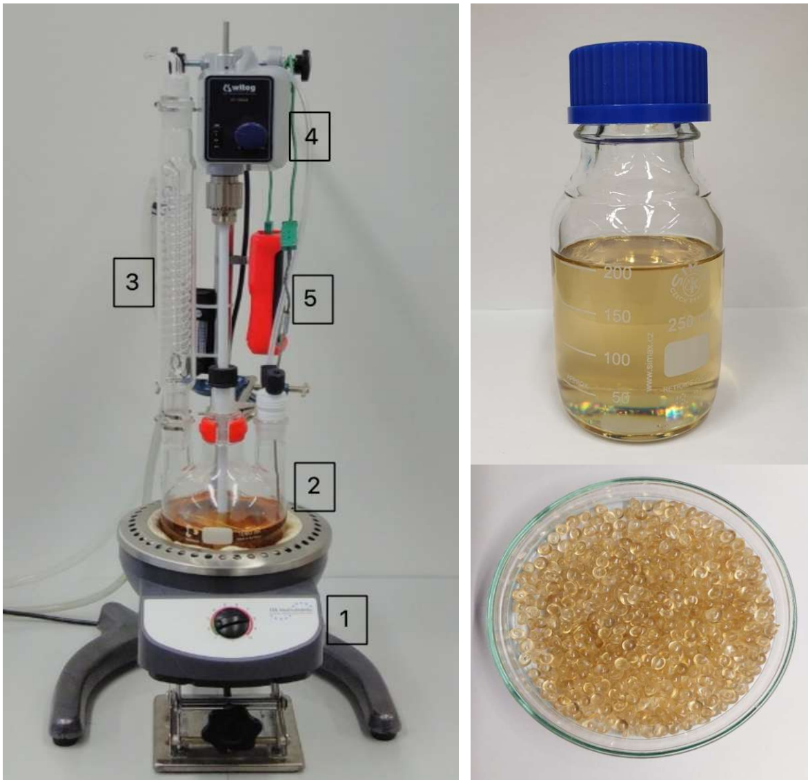
Figure 28: (a) Dope solution production process: heating mantle (1), triple-necked round-bottom flask (2), Dimroth condenser (3), Stirring motor (4), Thermolement (5) (left); (b) Polyethersulfone/1-methyl-2-pyrrolidone dope solution (top right); (c) Polyethersulfone pellets (bottom right)
