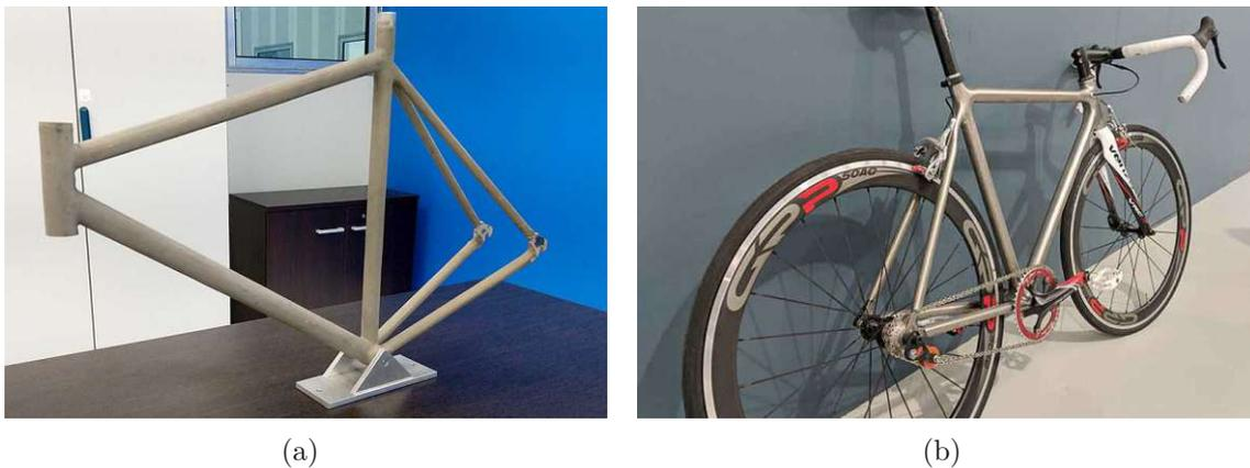
Figure 2.19: (a) Additive manufactured, seamless bike frame out of titanium; (b) bike with the installed bike frame, courtesy of Titomic Ltd. [31].
