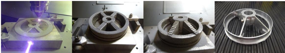
Figure 2.11: Productions steps of a fan frame for an UAV made of an aluminium alloy during the FFG project (Austrian Research Promotion Agency) *GenerAl* (FFG Nr. 843981), courtesy of the whole project-consortium [17].
