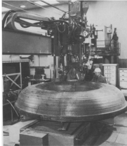
Figure 2.3: 3D printed half-toroid, after printing the part was cut apart and welded together to form a 180° pipe elbow [10].
