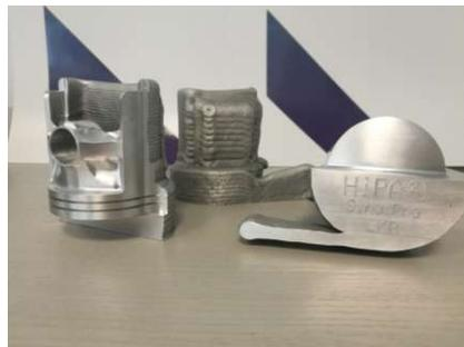
Figure 2.12: Additive manufactured piston made of aluminium, courtesy of LKR GmbH [19].
