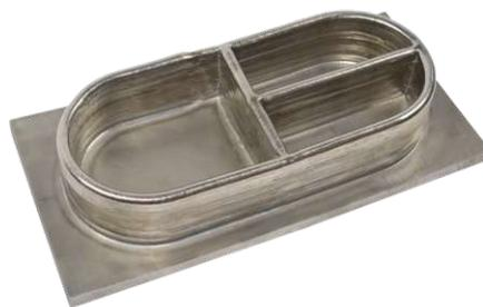
Figure 2.9: Titanium structure made by plasma arc DED process [15].
