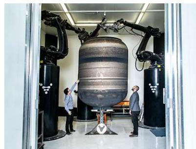
Figure 2.16: Relativity Space's AM-syste Stargate with printed aluminium tank [28].
