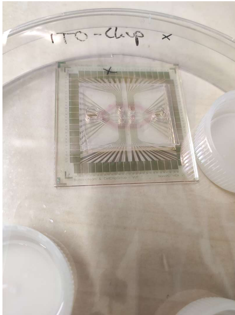
Figure 5.7: The loaded chip in petri dish before measurement (D9)
