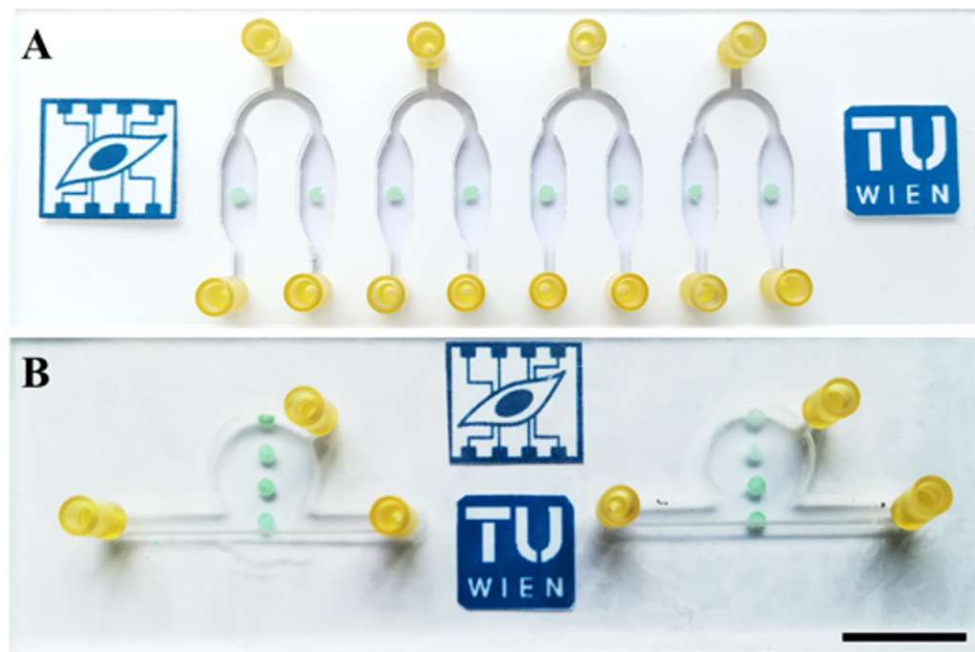
SI Figure 1: Images of microfluidic devices. (A) Microfluidic glass chip (76 x 76 x 2.3 mm) for monolayer culture containing 8 chambers with a sensor spot centralized in each chamber. (B) Microfluidic glass chip (76 x 26 x 4.4 mm) for three-dimensional (3D) hydrogel cultures with 4 sensor spots in each chamber. Scale bar represents 10 mm.
