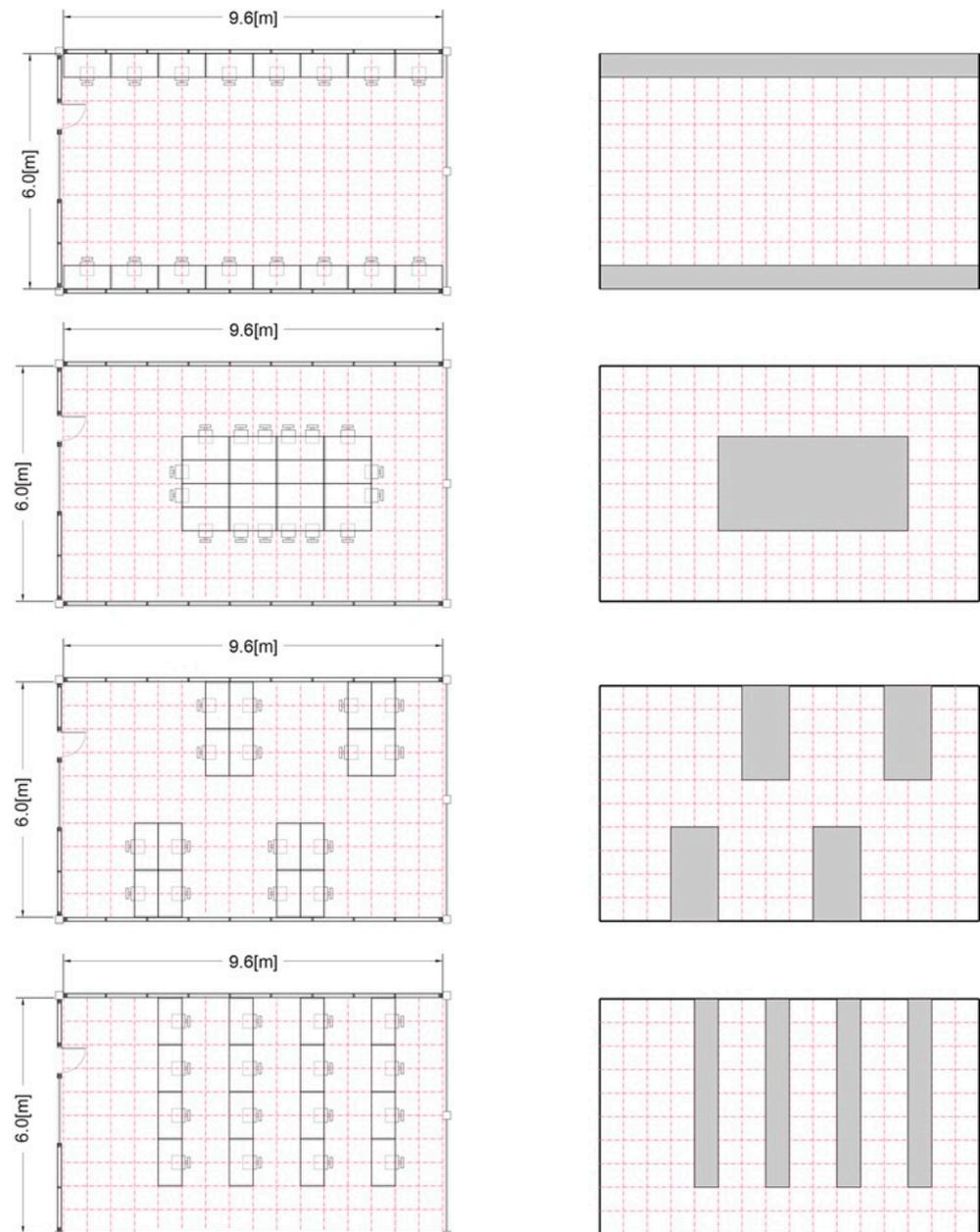
**Figure 1.** Floor plan and schematic representation of a typical classroom with four different furniture layouts.
