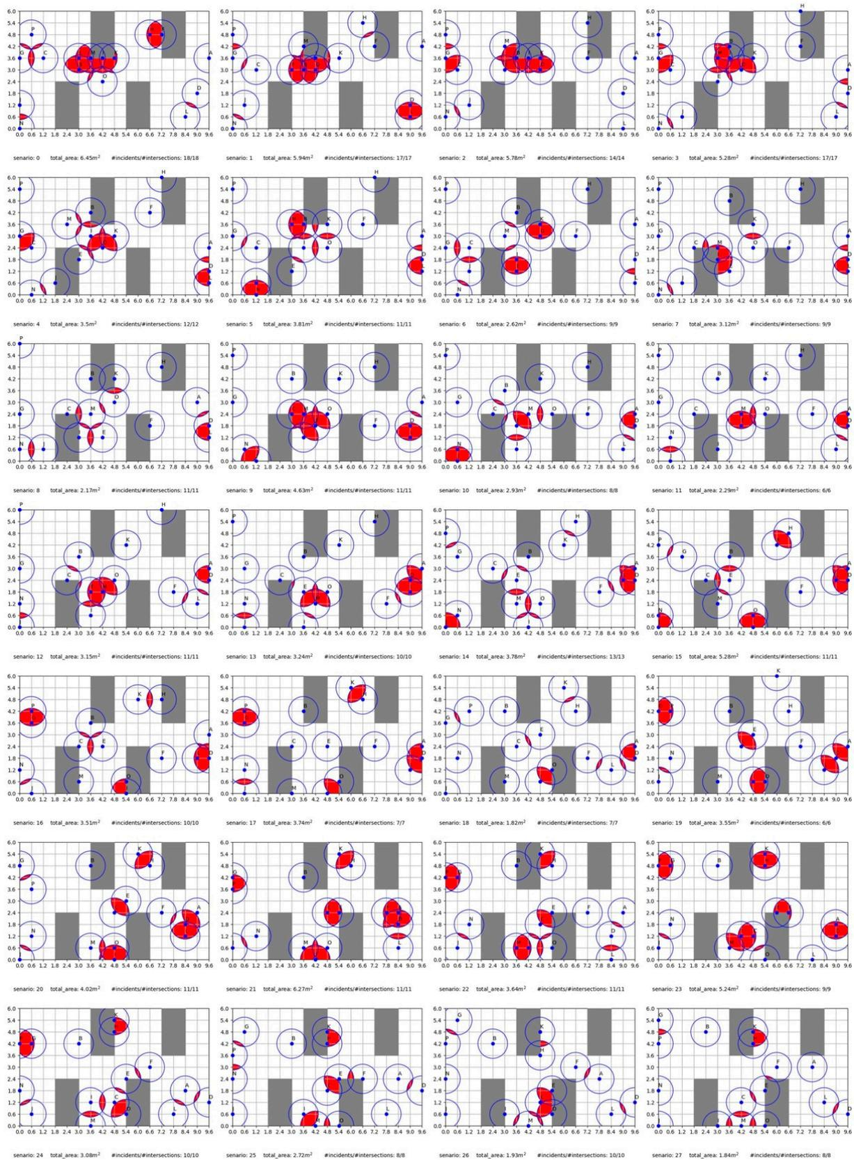
Figure 5. Graphic output showing simulated occupant positioning with the furniture layout for teaching and learning activity 3 (group work), without contact time consideration.
