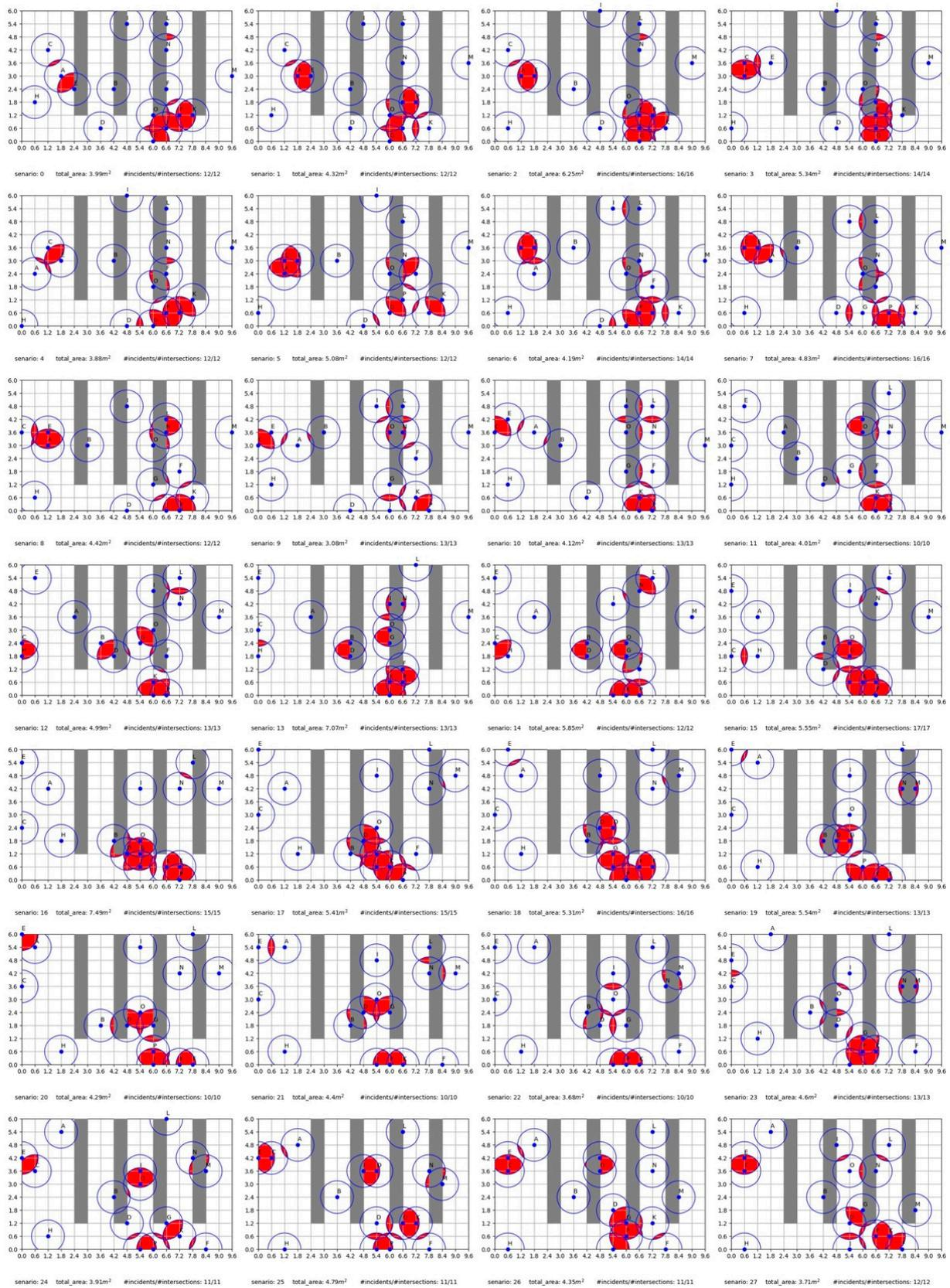
**Figure 6.** Graphic output showing simulated occupant positioning with the furniture layout for teaching and learning activity 4 (individual work), without contact time consideration.
