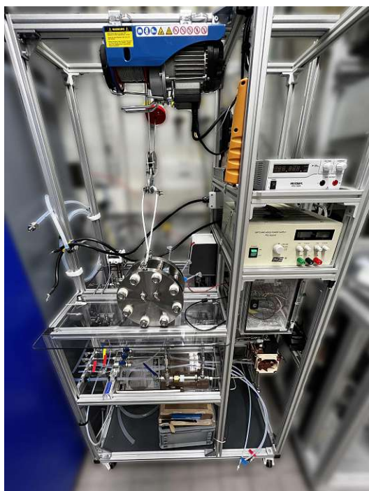
Fig. 3.1: Picture of the laboratory setup showing the thermostatic bath with the humidifier behind the compressor on the table (middle), the gas drying unit (bottom right), the temperature control & sensor electronics (middle right), the compressor power supply (middle right) and the power supply for the gas drying unit (top right)
