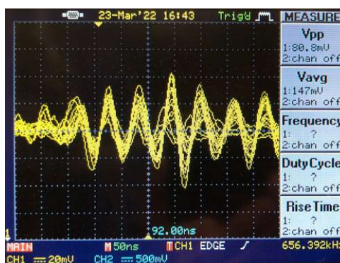
Fig. 5.1: The “PS900W” power supply set to 0,1 V DC is connected to an oscilloscope in parallel to the compressor as a load. The oscilloscope, set to 20 mV/division vertically, shows AC noise of about 80 mV peak to peak.
