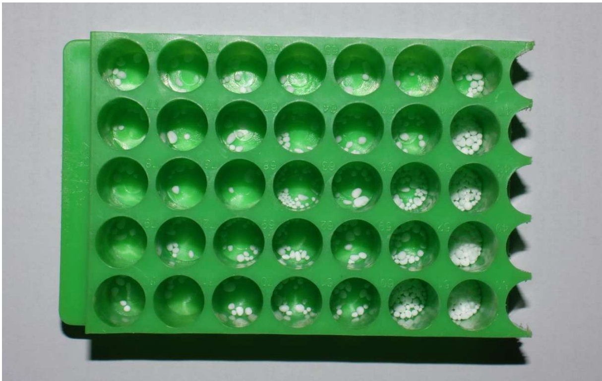
Figure 13: A picture of the vialplate used in this experiment. Each vial holds a defined amount of de-icing salt which will be used to determine the melting rate of this salt. This image shows that if the camera is positioned directly above the middle of the plate the cavities on the edges are not completely visible. This restricts the size of the plate.
