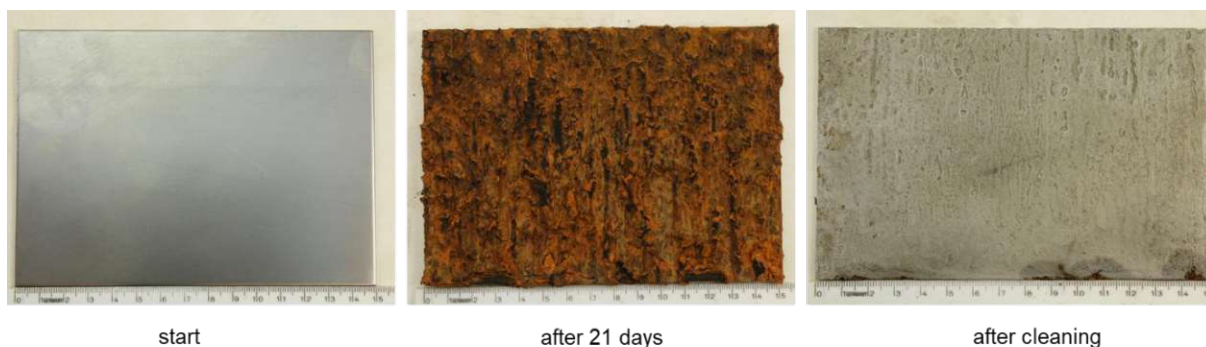
Figure 23: This picture shows the development of one Fe- plate during our corrosion process.
