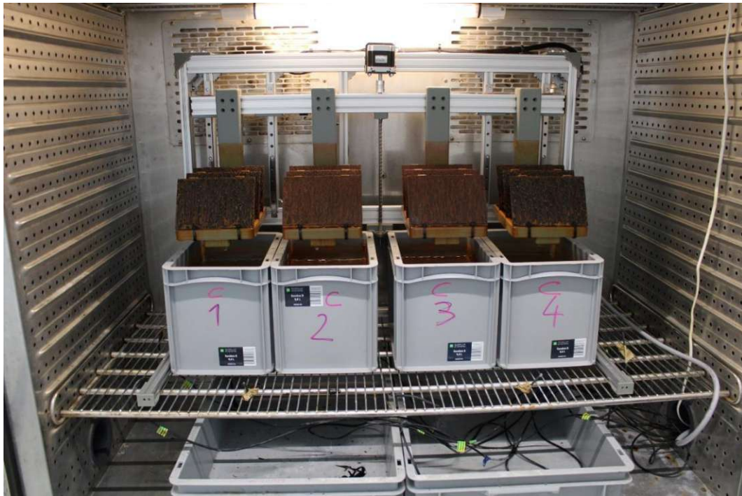
Figure 21: A picture taken of the final corrosion system. The grey containers are filled with different de-icing salt solutions. Every hour the sample plates are immersed into the solution for 10 minutes. Then they are lifted to give the oxygen time to corrode the metal.
