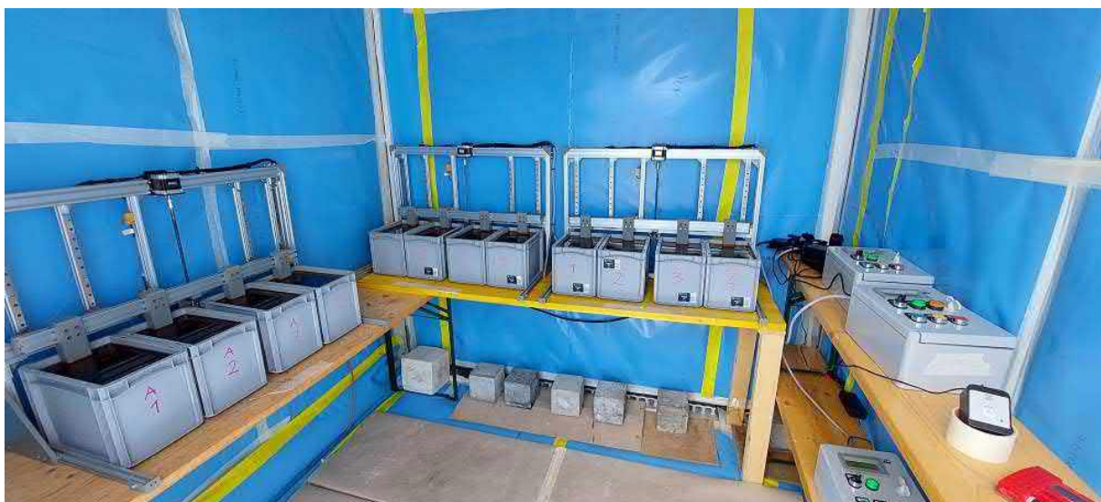
Figure 21: A picture taken of the final corrosion system. The grey containers are filled with different de-icing salt solutions. Every hour the sample plates are immersed into the solution for 10 minutes. Then they are lifted to give the oxygen time to corrode the metal.
