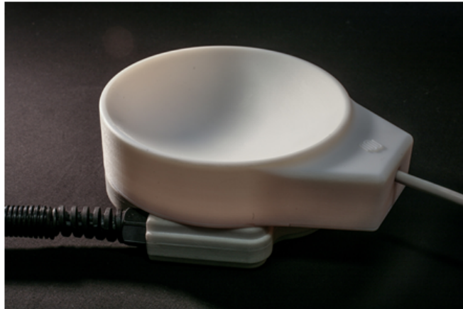
Figure 7.1.: Photograph of the custom 7 channel surface coil built in our lab.
