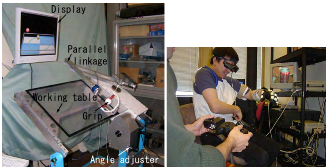
Figure 2.8: Left: PLEMO Rehabilitation System for Upper Limbs. The patient has to move the grip over the working table, according to the task, given on the screen [17]. Right: The user is wearing a HMD and a glove for interacting with a virtual environment [20].
