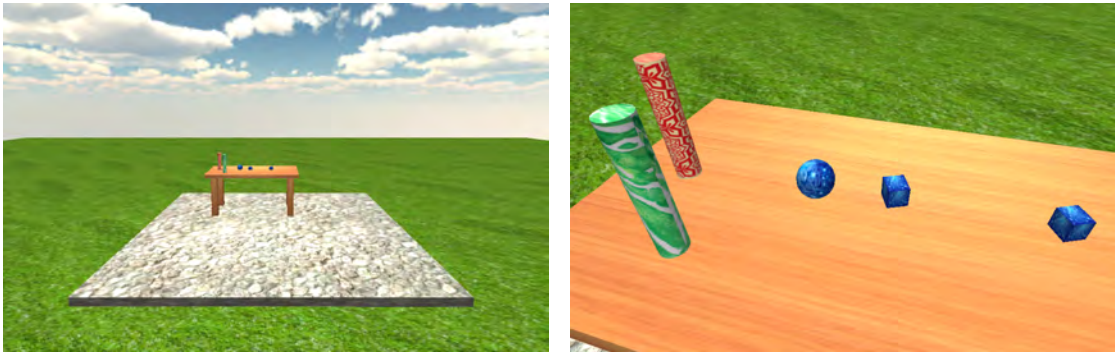
Figure 4.11: Left: The environment design, as it was used in the first part of the work. The task was to simply grasp the objects on the table by closing the virtual hand around them, and move them around afterwards. Right: The training objects used in this first design were shaped as cylinders, spheres and cubes.
