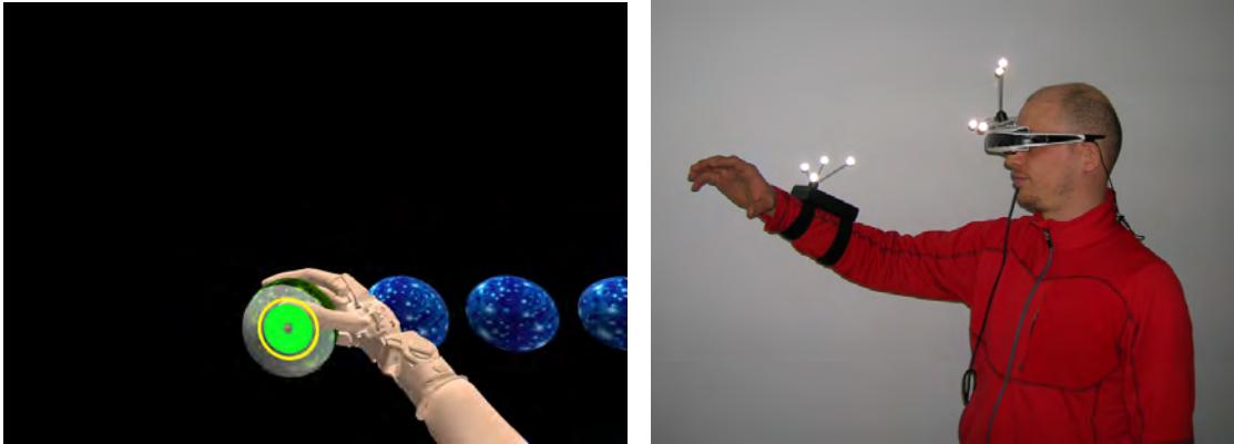
Figure 6.2: The Grasping in Motion scenario. The task of this scenario was to grasp and slightly move away the training objects before releasing them again. The objects were aligned in the shape of a circle, placed in the middle of the interaction (tracking) area.
