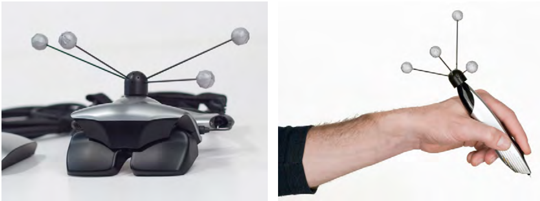
Figure 3.2: Two examples of ioTracker tracking targets, attached to a HMD (left) and a pen (right).
