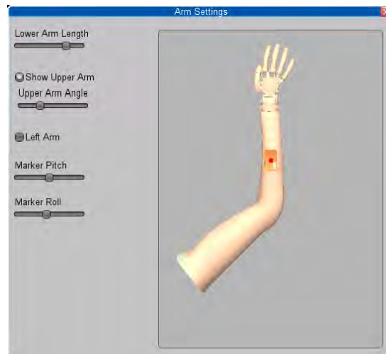
Figure 4.8: The Arm Settings Window displaying a virtual illustration of the tracking target. The target can be moved and rotated to be placed anywhere on the arm.
