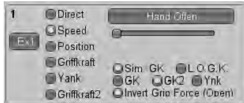
Figure 4.10: Options for simulating Grip Force at one mapping. Ex1 means, that the first one of the incoming EMG signals is used as an input.
