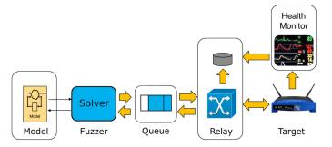
Fig. 4. An overview of a hardware-in-the-loop fuzzing architecture
