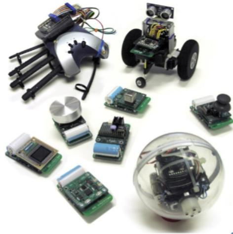
**Figure 2.5:** A Wide Field of Sun SPOT Applications: Robots, Remote Controls and Cybernetic Devices such as an Electronic Glove. Source: [ORACLE, 2012b].
