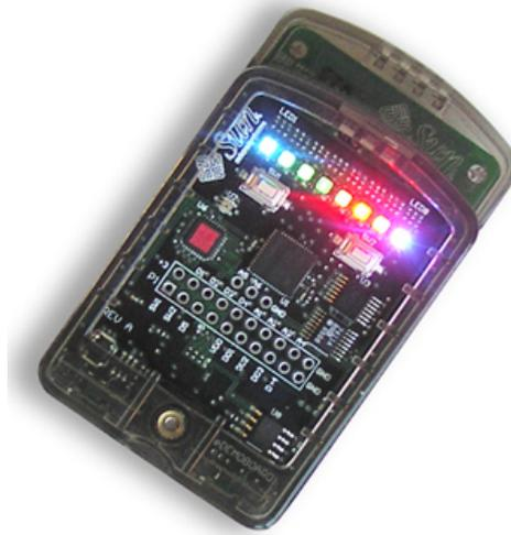
**Figure 1.3:** Sun SPOT from ORACLE. Source: [ORACLE, 2012b].
