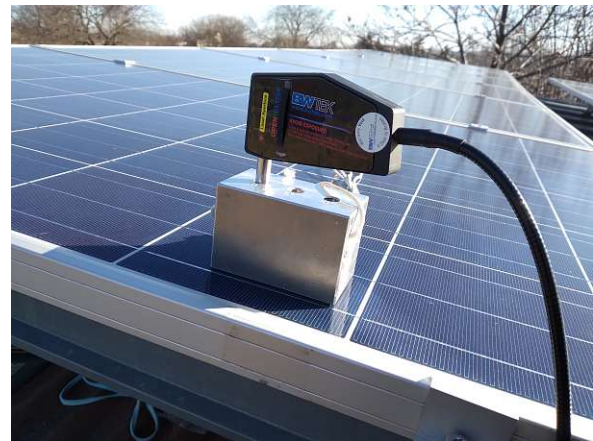
(b) Laser probe measuring the encapsulant of the modules using a specially designed spacer.
