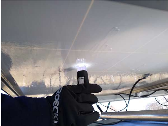
(a) Measurement with the light microscope on the Remsolar-coated backsheet of Module 1.
