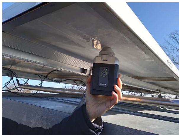
Figure 4.11: Measurement with the NIR-spectrometer on the Remsolar-coated Module 1.
