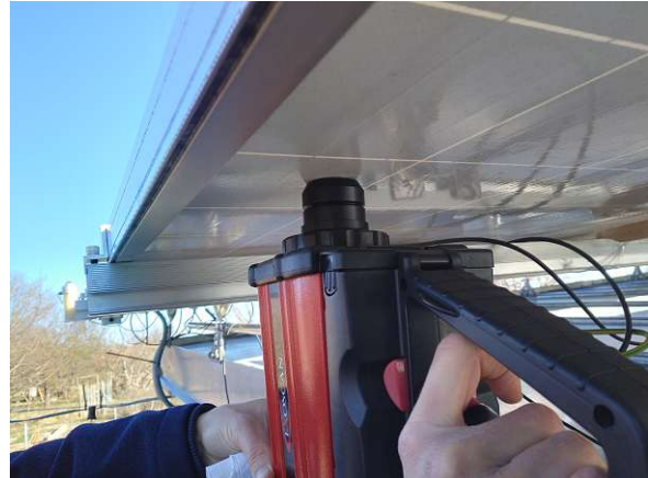
(b) Measurement with the EXOSCAN FTIR-spectrometer on the Dowsil-coated backsheet of Module 7.
