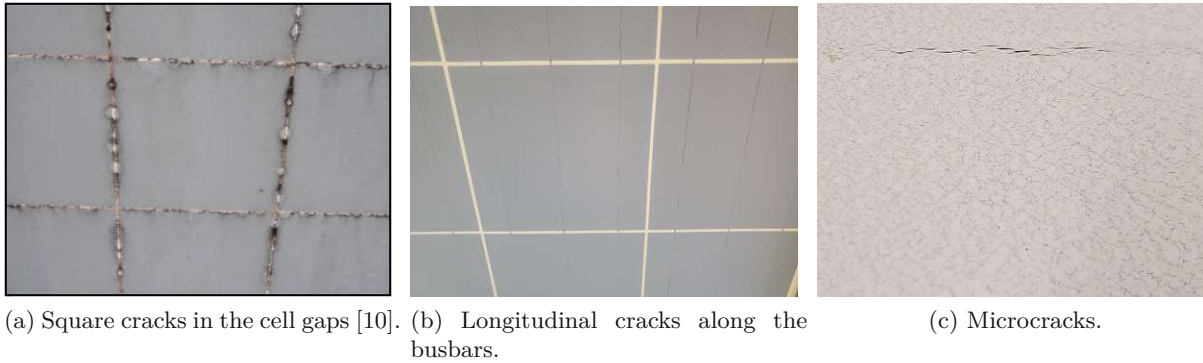
Figure 1.2: Different crack types in polyamide (PA) backsheets.
