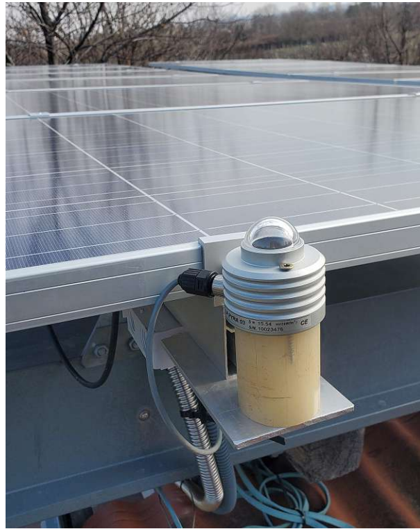
Figure 4.4: LP PYRA 03 pyranometer mounted next to Module 1, parallel to the module plane (plane-of-array irradiance), with the test site in the background.
