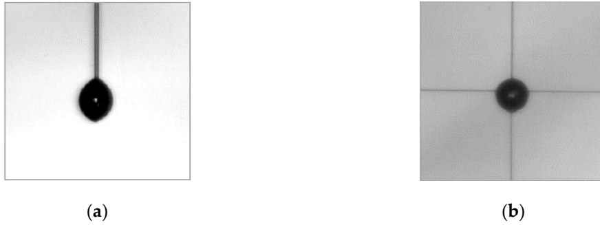
Figure 6.2: Droplet suspending techniques (reprinted from [96]). (a) Nomura [97], (b) Chauveau [96].
