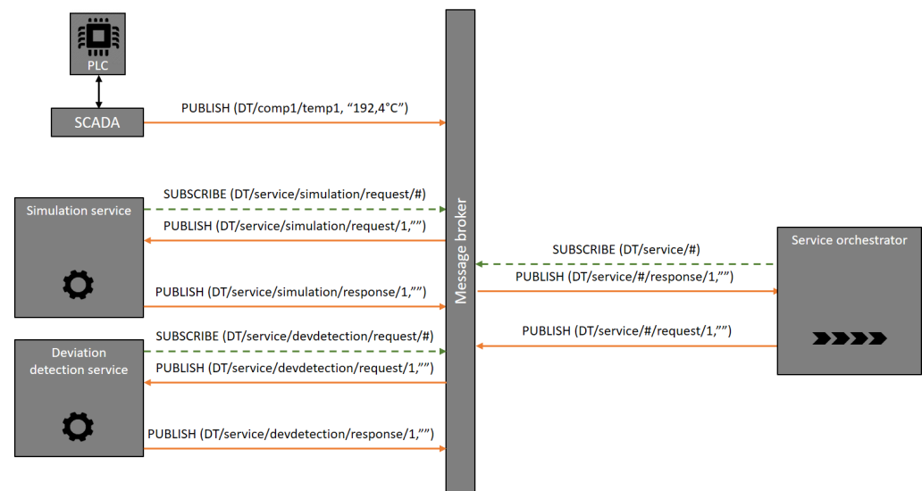
Figure 3. Exemplary request–response message pattern in the DT platform. Services subscribe to their respective request–topics and thereby receive messages published by the service orchestrator, e.g., to start operating. When a service instance has completed a run, it publishes to its response topic, which is monitored by the service orchestrator via subscription. Note: The function of the service orchestrator is explained in detail in Section 3.5. Character # denotes a multi-level wildcard, hence receives all messages of a topic that begins with the pattern before the wildcard character, and " " contains message payloads.
