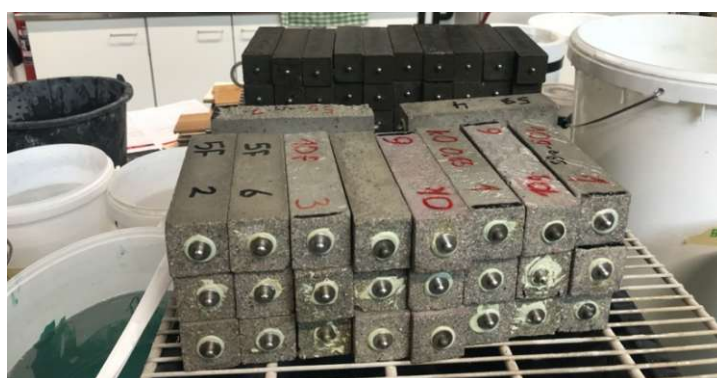
Figure 12 Mortar prisms (F and B) in the oven exposed to the wetting cycles (60°C)
