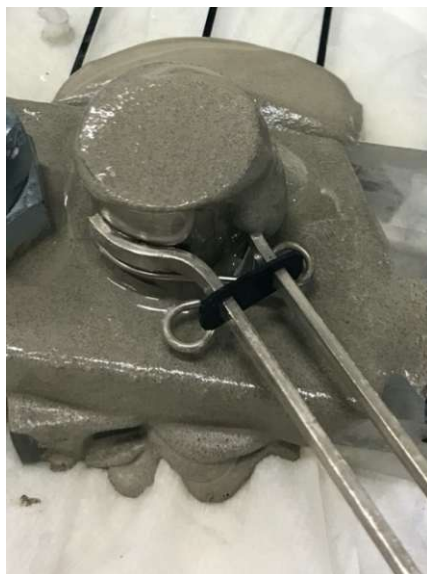
Figure 42 low consistency of hydrated Fondu (HF)
