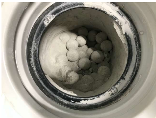
Figure 8 The result of the milling and the ceramic balls
