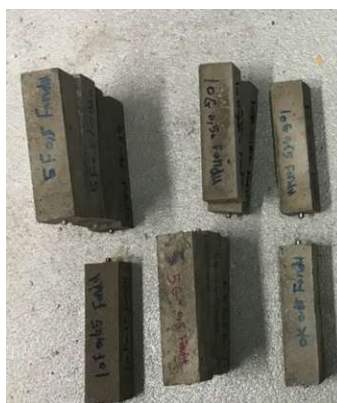
Figure 10 Mortar prisms of fresh cement Fondu (F)
