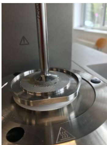
Figure 15 sample of cement slurry during the rheological tests
