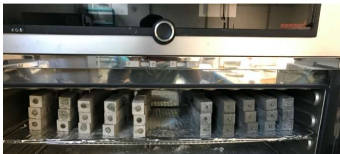
Figure 11 Mortar prisms (F and B) in the oven exposed to the heating cycles (60°C)
