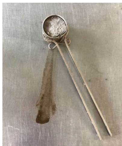
Figure 43 Degradation of hydrated Fondu (HF)
