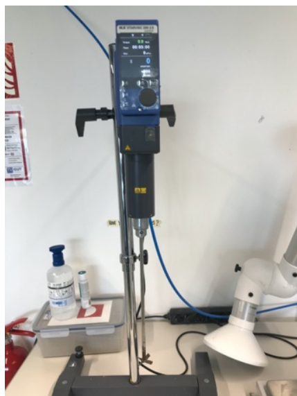
Figure 16 Mixer used for preparing LC samples
