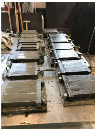
Figure 6 Cement paste casting to prepare the hydrated cements
