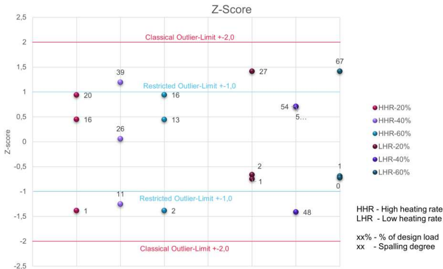
(d) Z-Score for HSC half scale columns under low and high heating rate - every dataset calculated individually
