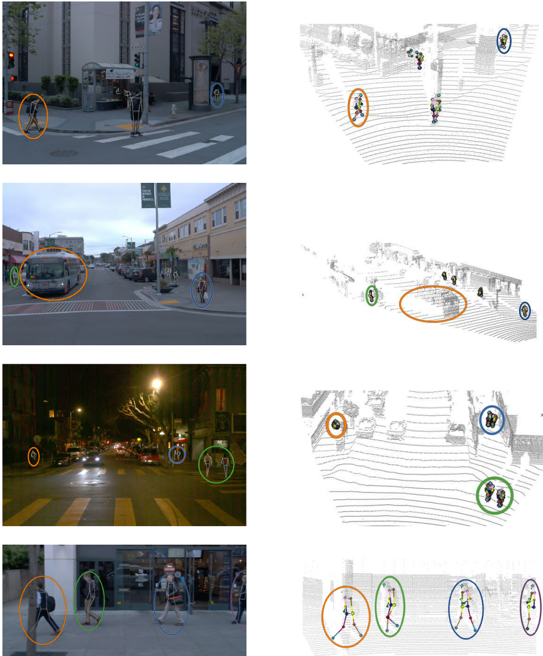
Figure 3.7: 2D and 3D pseudo-labels visualized on four selected scenes from the WODS++ development set. Colored ellipses mark corresponding objects in image and point cloud to aid orientation. Each keypoint type has a different color, consistent across people.
