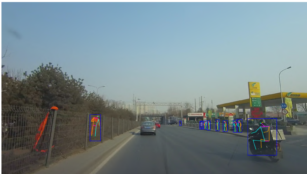
Figure 2.3: Sample image with pose labels from TDUP. Reproduced from [WYW + 21]. Colors distinguish left, right, torso and head keypoints.
