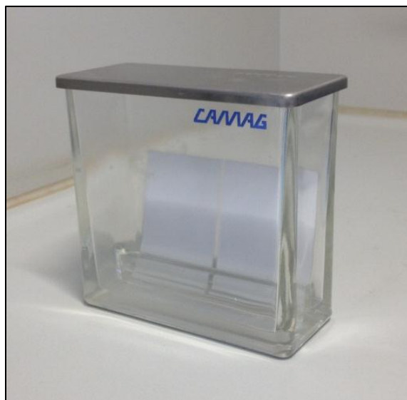
Figure 11: Twin trough chamber from CAMAG used for HPTLC analysis.
