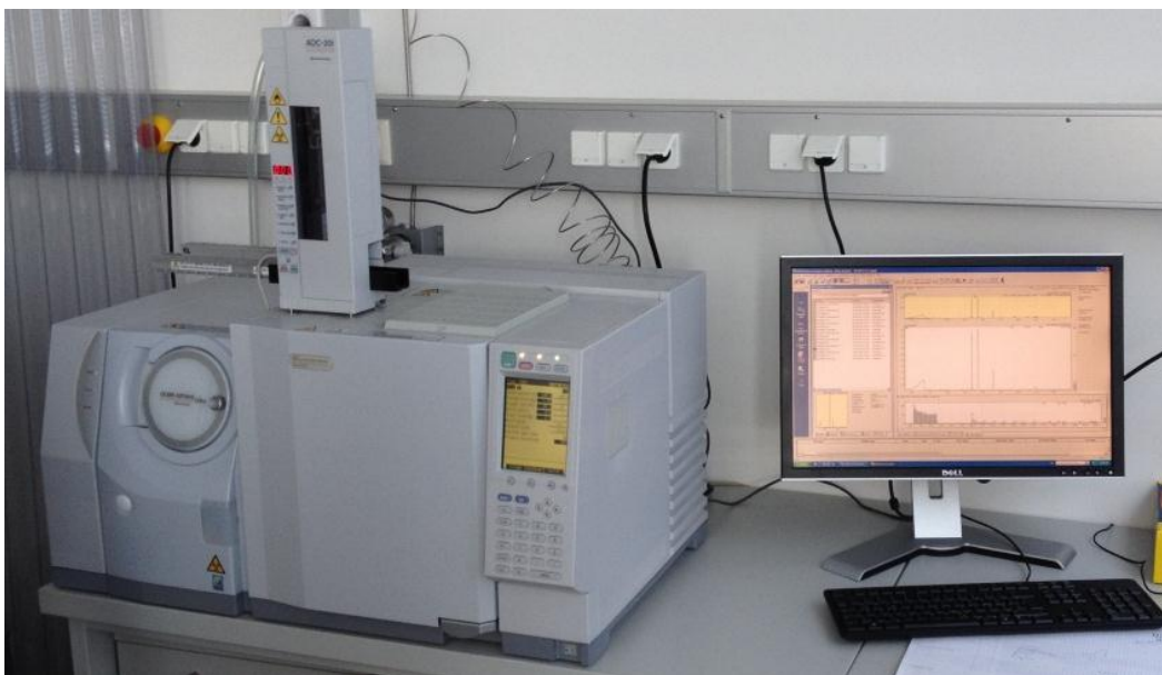
Figure 14: Picture of the GCMS from Shimadzu and the connected PC
