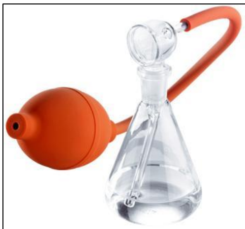
Figure 12: Reagent sprayer used for staining the HPTLC plates and detecting the sample bands [22].
