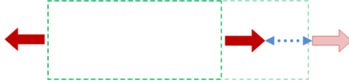
Figure 4.19: Dragging a scale-arrow should look for the user as if he drags only one side of the box.
