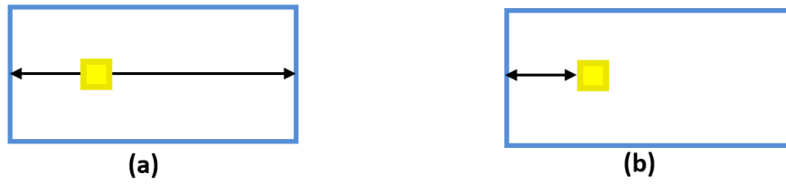
Figure 4.3: Binary relations, marked by yellow boxes, can be oriented relatively between two sides of the box (a) or with absolute offset to one side (b). The arrows show to which sides of the bounding box the binary relation is related.
