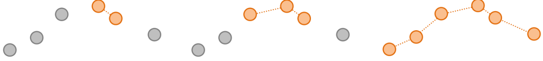
Figure 4.14: The greedy algorithm for control-polygon generation: (Left) Initial polygon, (Middle) Nearest point is joined to the polygon, (Right) Final polygon.
