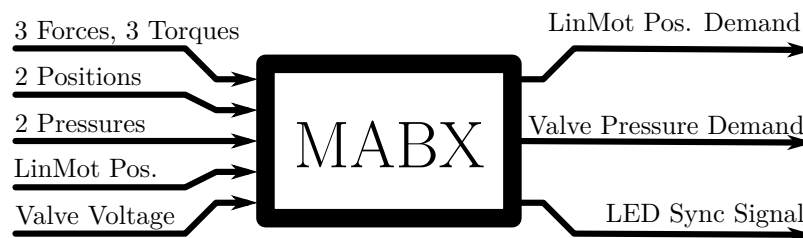
Figure 3.2: Signals processed by the MicroAutoBox II (left: Sensors, right: actuators)
