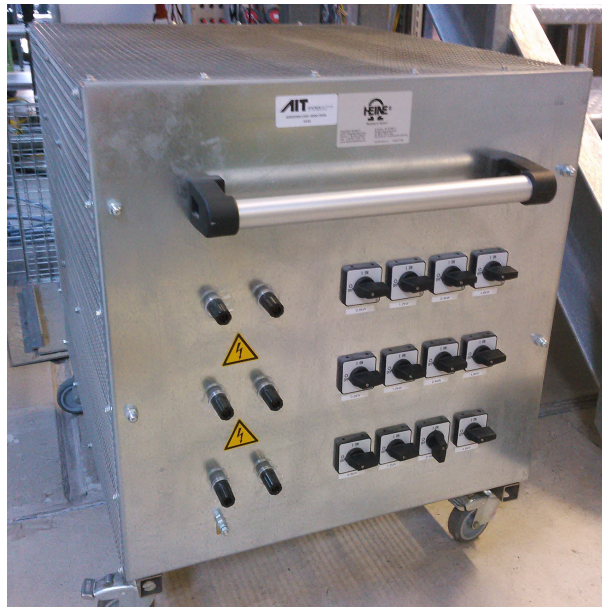
Figure A.1: Picture of the manually switchable AC load
