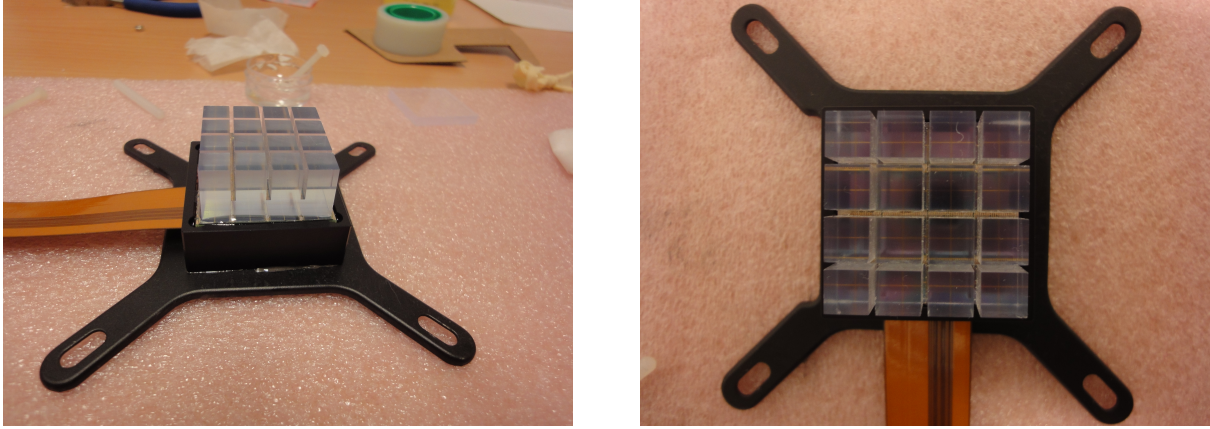
Figure 8.24: Pictures of the segmented BC-408 plastic scintillator attached to a DPC-3200. The geometry of the scintillator has been adapted to the layout of the DPC to achieve position resolution. The slits are 1 mm wide and 10 mm deep and fit the regular die pattern of the DPC. This scintillation detector was used as a reference counter.
