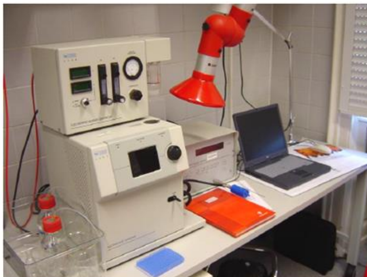
Figure 2.1: Photo of GEMMA instrument at TUVIE
