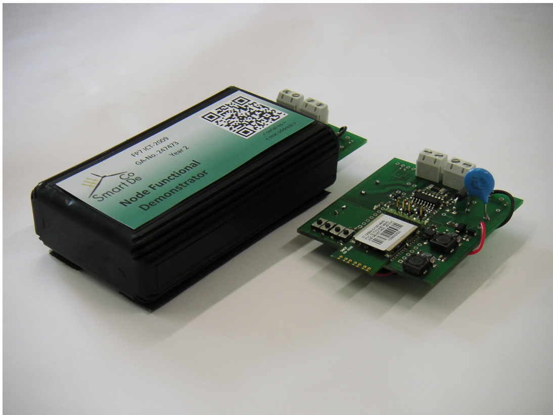
Figure 7.2: Picture of a SmartCoDe node and its casing.
