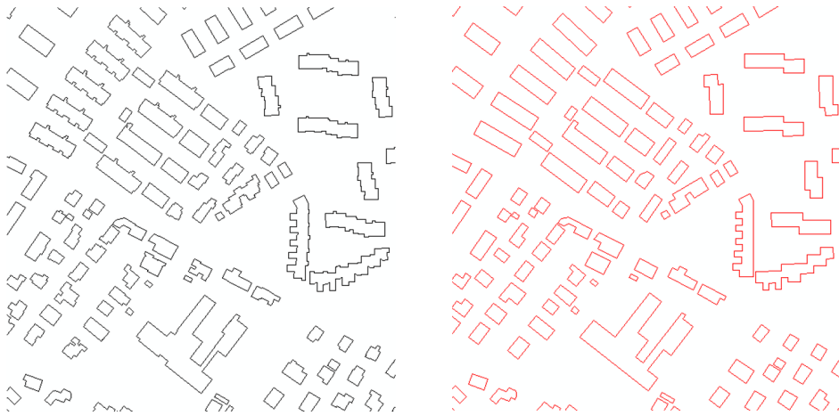
Figure 4.4: The result of the operator Simplify Building is represented on the right
