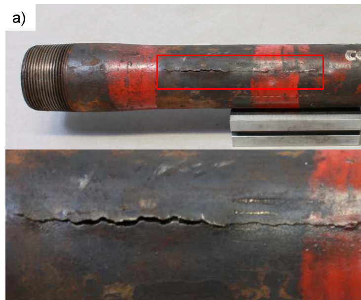
Fig. 5.1: Local wear damage on the carbon steel tube, which was used in real application, seen outside as crack [cf. 74]
