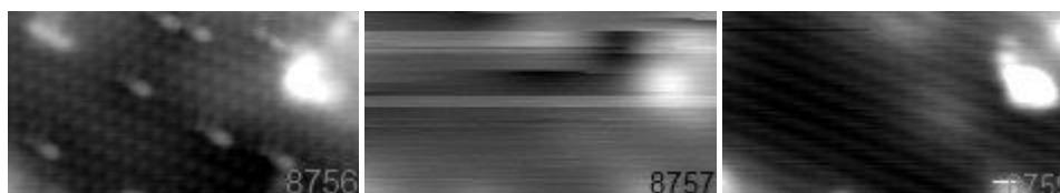
Figure 19: 8 \times 4 \text{ nm}^2 , 1 V, 0.1 nA, water (0.015 L, 3.2% coverage) was converted into bridging oxygen dimers (left image) by a prior 4 V scan. These are removed by a 5 V scan in the middle image.
