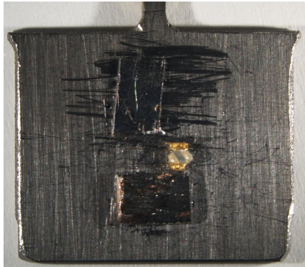
Figure 11: Photograph of the synthetic sample mounted on an 18 \times 15 \text{ mm}^2 omicron Ta sample plate. The materials used for the holder are Ta and Au.
