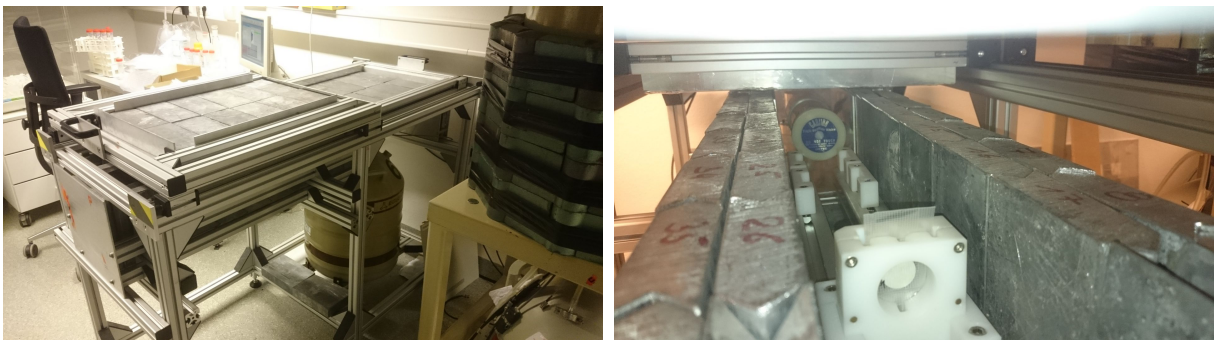
Figure 19 The current setup is pictured on the left side. The right image shows an inside view of the setup. The sample is mounted in the front, the detector window is visible in the rear.
