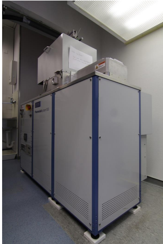
Figure 18: Photograph of the Oxford Plasmalab 100 System used for the ICP-CVD silicon nitride deposition experiments. A schematic drawing is provided in section 2.2.3.
