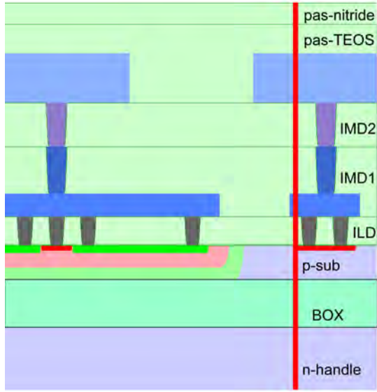
(a) Cross section schematics with optical path for the simulation indicated in red.
