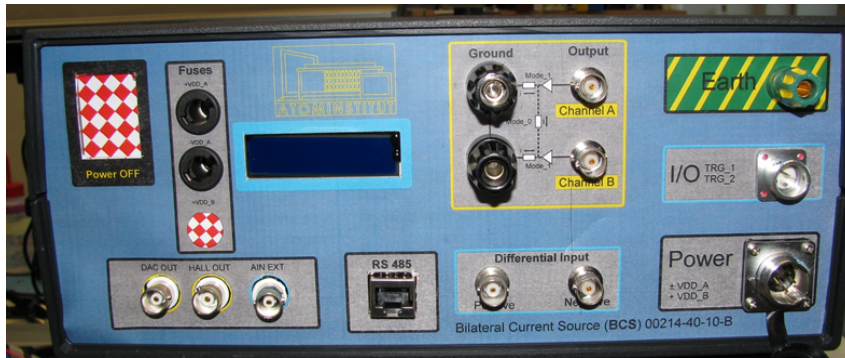
Figure B.4.: The front panel of the new current source. Programming the waveforms is done through the RS 435 socket. DAQ out and Hall out allow analog monitoring of the current setting, all other parameters can be read through the programming interface.
