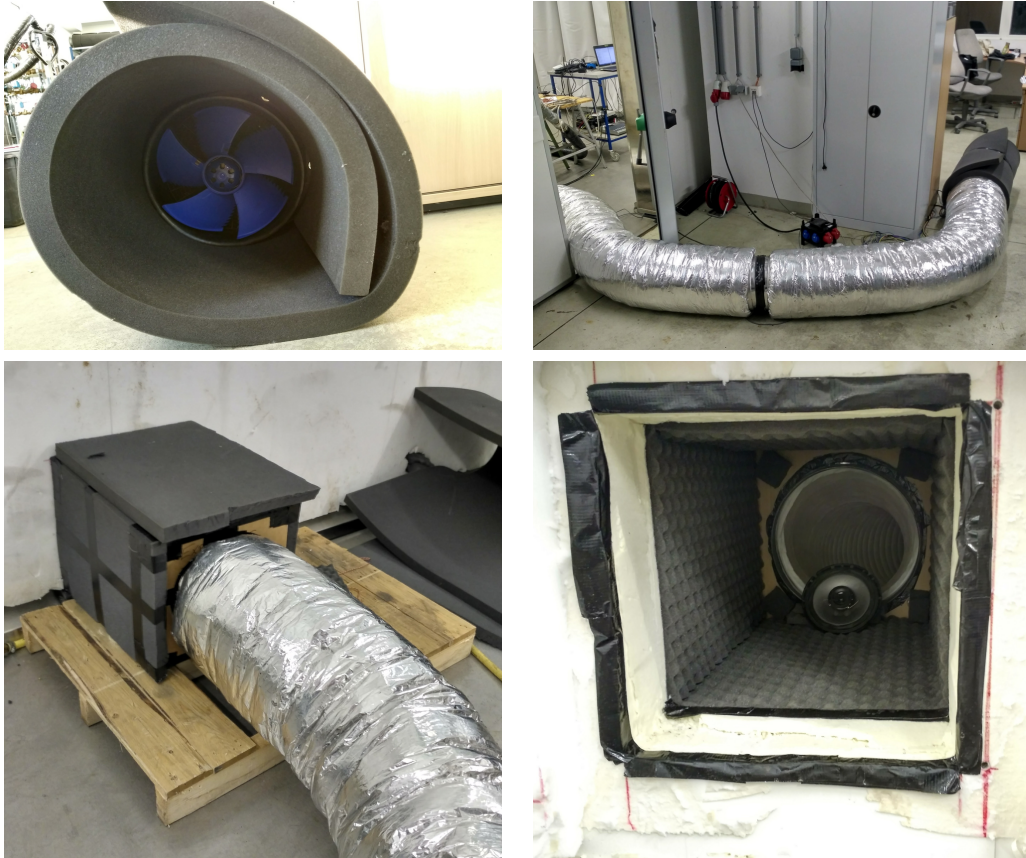
Figure 24: Path of the air flow. Top left: Fan, rolled up into a thick piece of sound absorbing material. Top right: Flexible insulated air duct, entering the climate chamber. Bottom left: Round-to-square adapter box, with sound absorbing material on inside and outside. Bottom right: Wall opening, seen from the second climate chamber.
