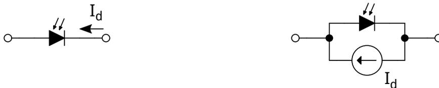
(a) Photodiode circuit symbol with an arrow indicating the direction of the photocurrent
