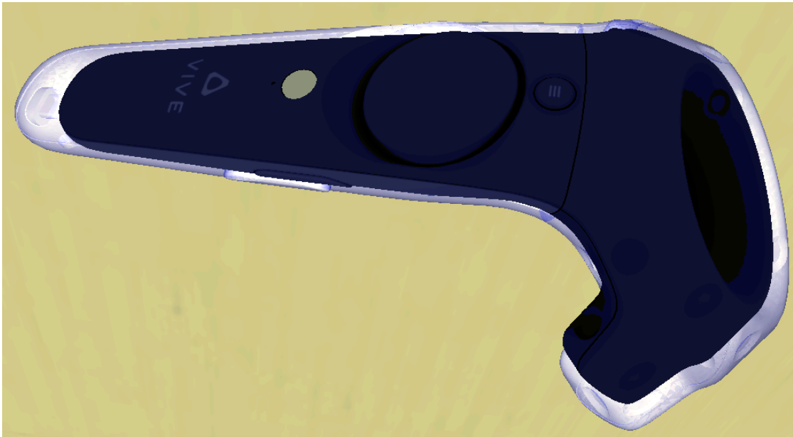
Figure 3.10: The transparent blue model is a visualization of the grabbing volume. The balls can be grabbed when they intersect with this volume. If the user fails to do so, the 'real' black controller can push the balls away.
