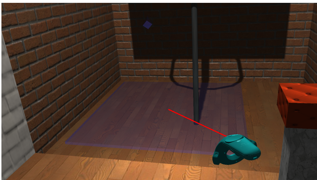
Figure 3.8: The blue field represents the tracking area after the teleportation. This makes it easier for users to make plans but can decrease the presence.
