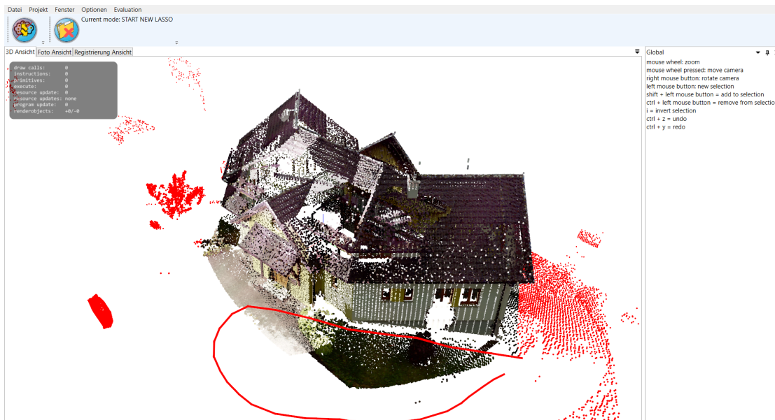
Figure 3.11: The point cloud is rendered in the central part of the window. The controls are described on the right. The menu allows users to load point clouds and start the comparison. The red points are already selected. The points enclosed by the red line will be selected, too.
