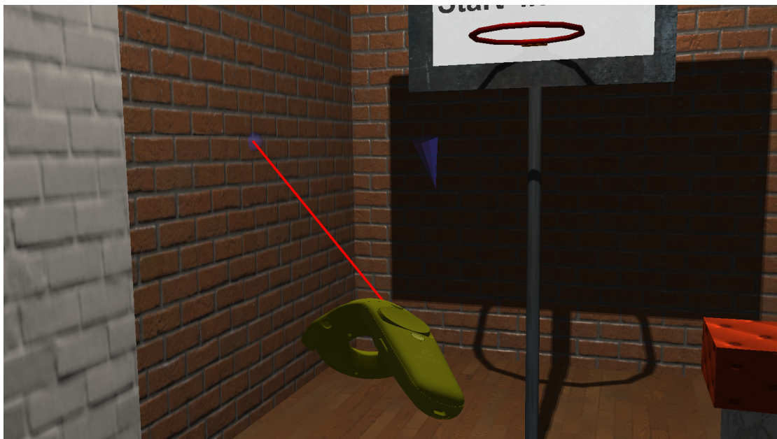
Figure 3.7: The blue cone represents the HMD after the teleportation. When using a ray-cast hit point as the target position, users cannot leave such a closed in-door scene.
