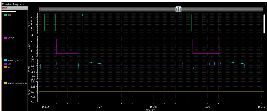
Figure 3.12: Example for the functionality of the digital checker
