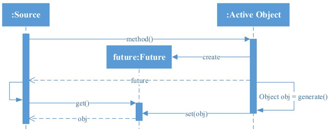
**Figure 3.1:** Sequence diagram of the asynchronous call mode using a future for result access.
