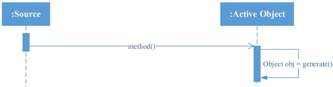
**Figure 3.2:** Sequence diagram of the purely asynchronous call mode.
