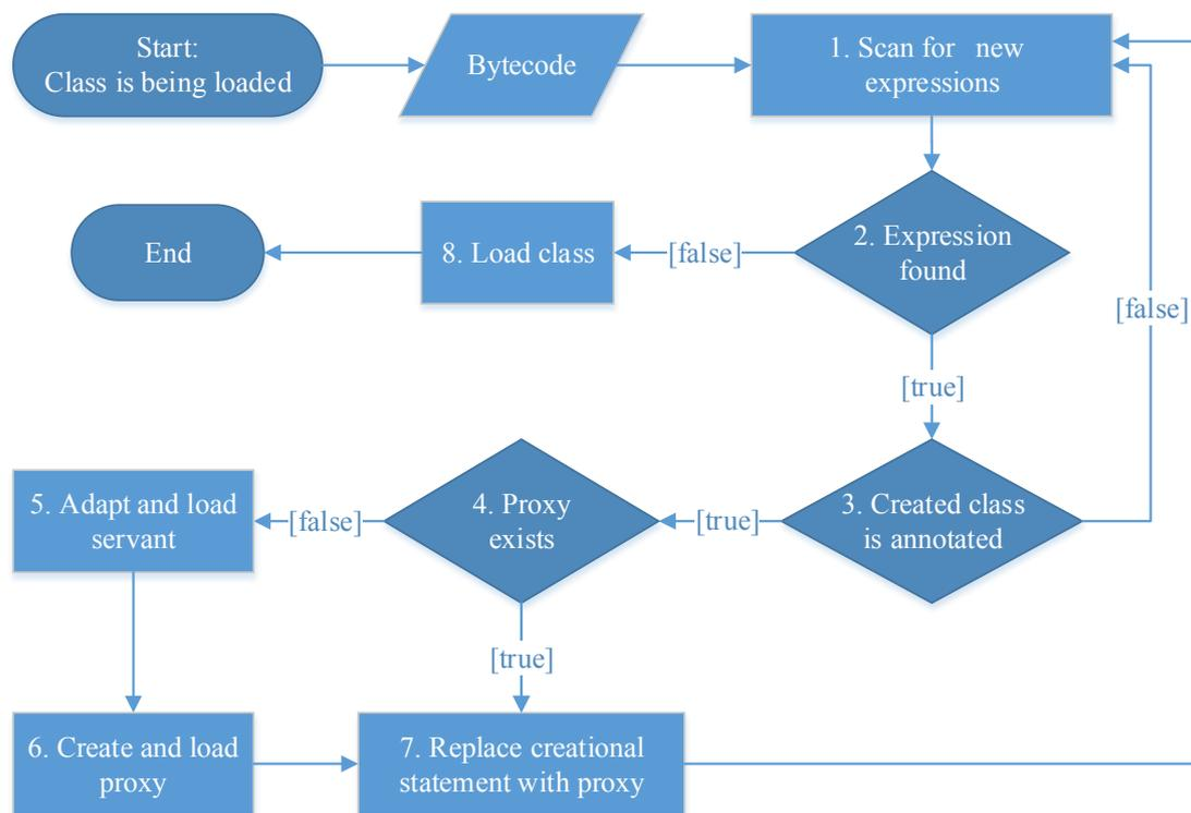
**Figure 5.3:** A high-level view of the approach chosen for the instrumentation.
