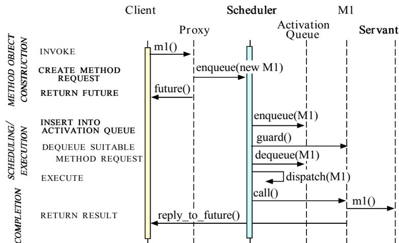
**Figure 2.4:** Sequence diagram of the different phases of an active invocation. [31]
