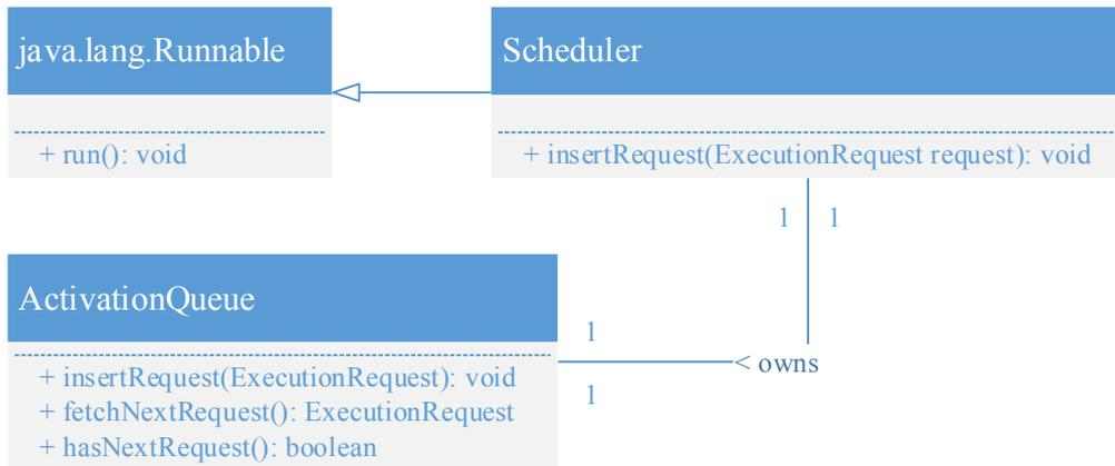
**Figure 4.3:** Class diagram of the scheduler and activation queue interfaces.
