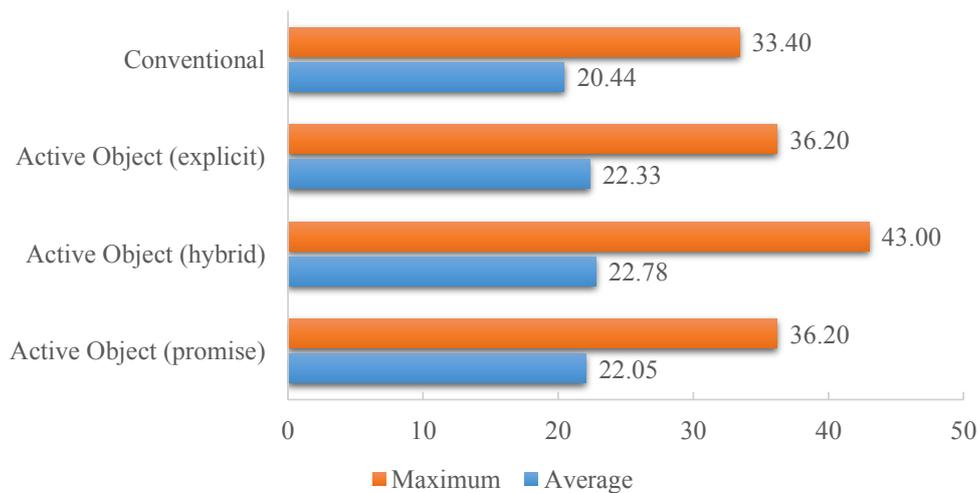
**Figure 7.5:** The average and maximum memory consumption of the approaches during the throughput run given in megabytes (lower is better).
