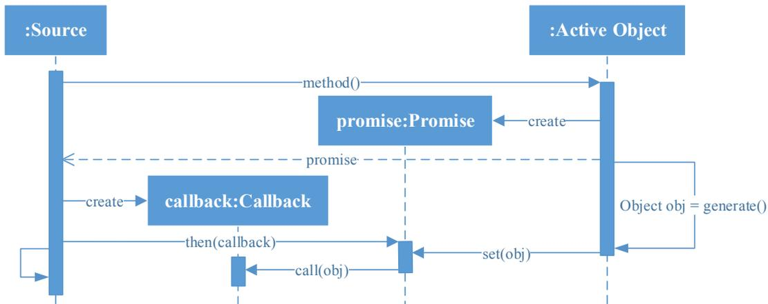
**Figure 3.4:** Sequence diagram of the asynchronous call mode based on a promise and a callback for result access.
