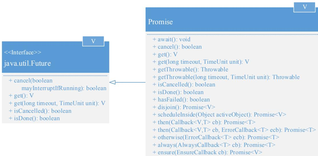
**Figure 4.2:** Class diagram of the modelled promise interface.
