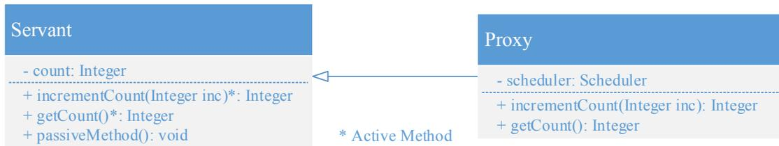
**Figure 4.4:** An example of a concrete proxy.
