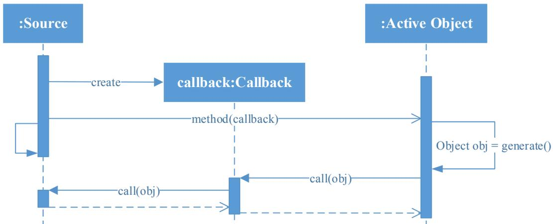
**Figure 3.3:** Sequence diagram of the asynchronous call mode based on a callback for result handling.
