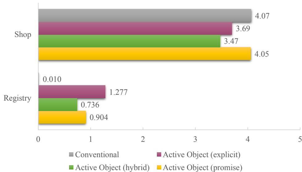
**Figure 7.3:** Average response time of the applications in milliseconds during the timed run (lower is better).
