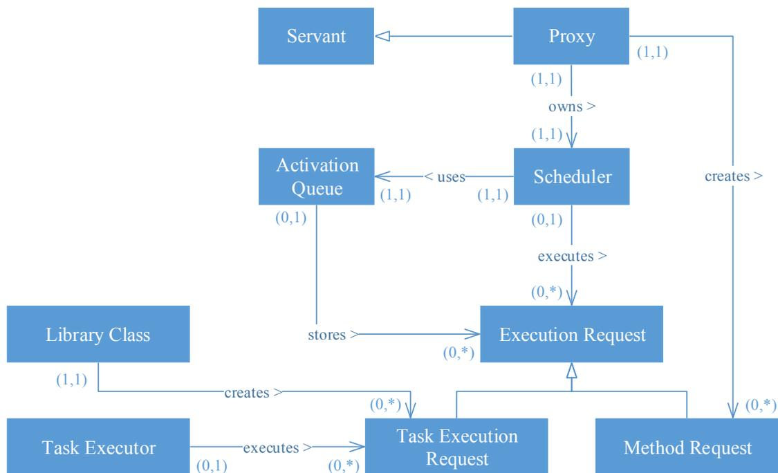
**Figure 4.1:** Class diagram depicting the relationships between the different core components.
