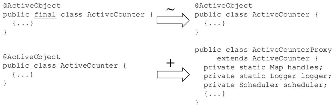
**Figure 5.4:** A number of code transformations necessary for the creation of the proxy class.
