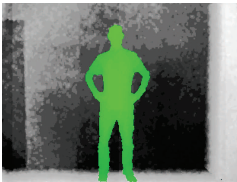
Figure 3.7: Automatic user segmentation in a captured depth image, provided by the NiTE middleware.
