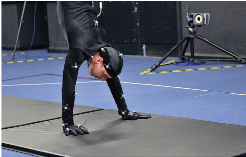
Figure 2.1: The optical motion tracking system VICON while tracking the motions of an actor wearing a suit equipped with passive markers. Image taken from 1 .
