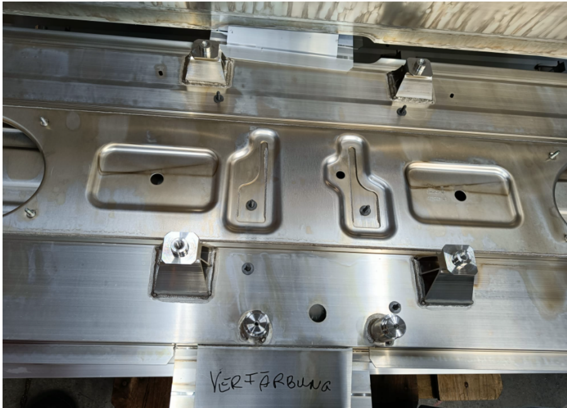
Figure 6.4: Company B - Aluminium brown stains coloration defect.
