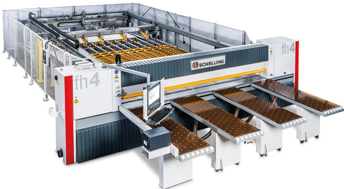
Figure 1.1: A cut-to-size saw for the wood cutting industry. (Image by SCHELLING Anlagenbau GmbH)
