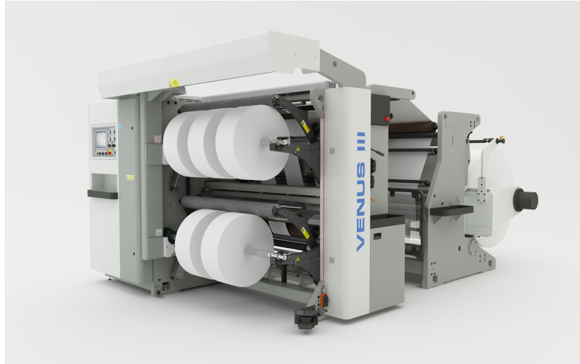
Figure 2.1: A roll slitting machine which cuts paper rolls into smaller rolls. (Image by Soma Engineering is licensed under CC BY-SA 3.0)
