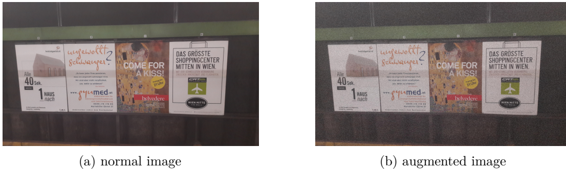
Figure 4.10: The effect of adding salt&pepper noise and a Gaussian blur to an input image.
