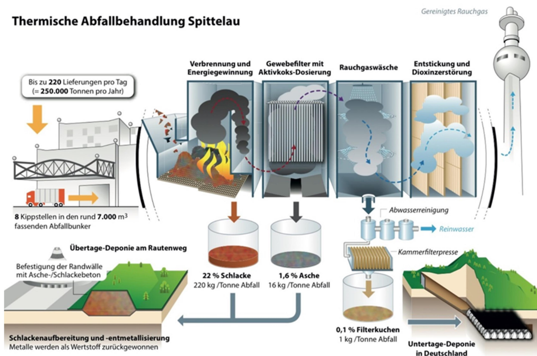
Figure 8 Thermal waste incineration application in the Spittelau, Wien, Austria
