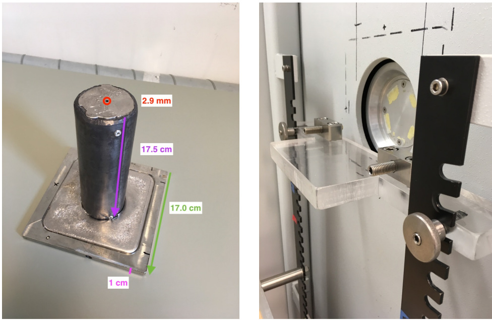
(a) The in-house built collimator has following dimensions: quadratic end-plate side length (green) = 17 cm, end-plate thickness (pink) = 1 cm, length (purple) = 17.5 cm, and opening hole diameter (red) = 2.9 mm
