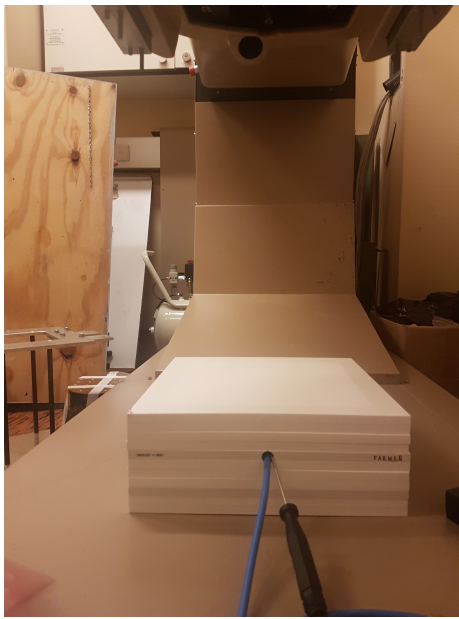
(a) The setup for calibration of the Farmer Chamber
