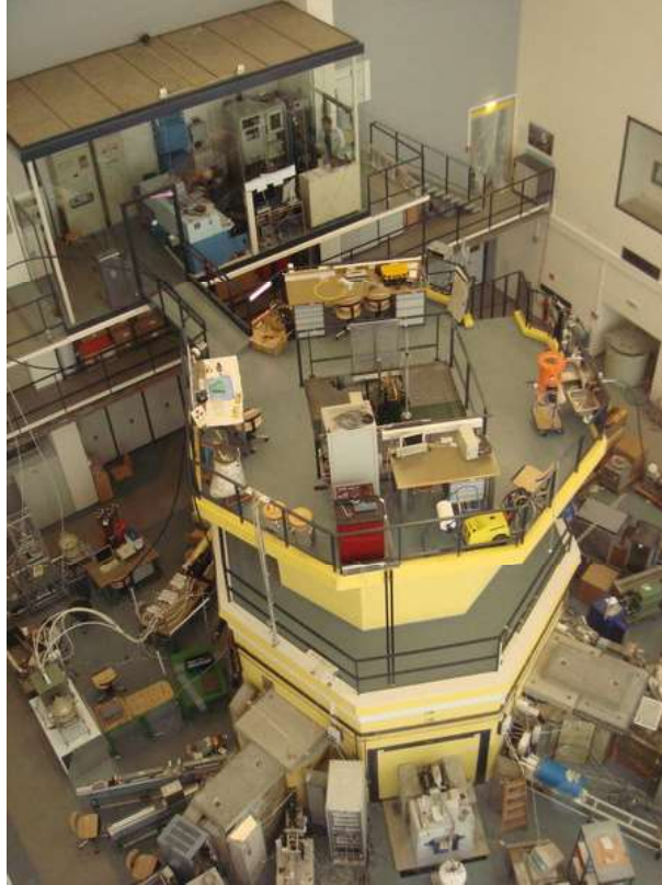
Figure 3.1: TRIGA Mark II Reactor in Vienna in the yellow coloured containment and different beam ports around it where free neutrons are used for experiments. (Photo from Section “Photos” in [28].)
