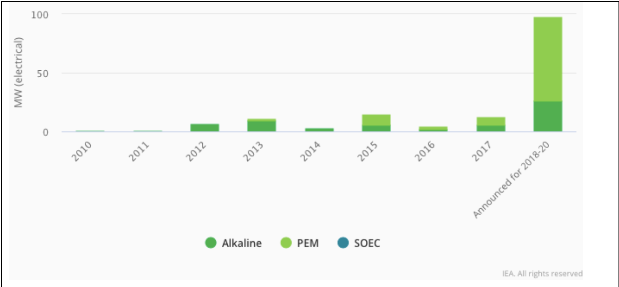
Figure 10. Global water electrolyser additions for energy applications by technology type. Source: (International Energy Agency 2019)
